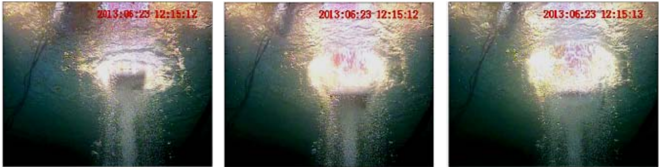
Fig. 11: Underwater oblique view of the impact ( \beta = 1.0\% , v = 4.09 m/s, m = 32 kg).
