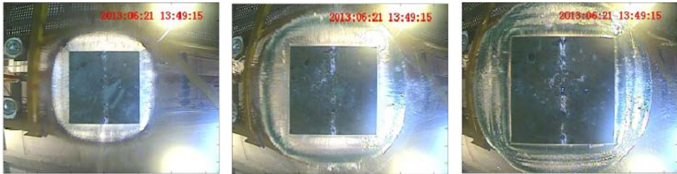
Fig. 9: Bottom view of the impact ( \beta = 0\% , v = 4.14 m/s, m = 32 kg).
