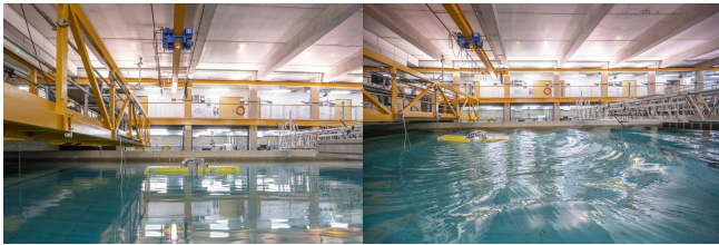
Fig. 2: COAST lab: pictures from Coastal, Ocean and Sediment Transport lab at the University of Plymouth to represent the conditions for an offshore turbine.
