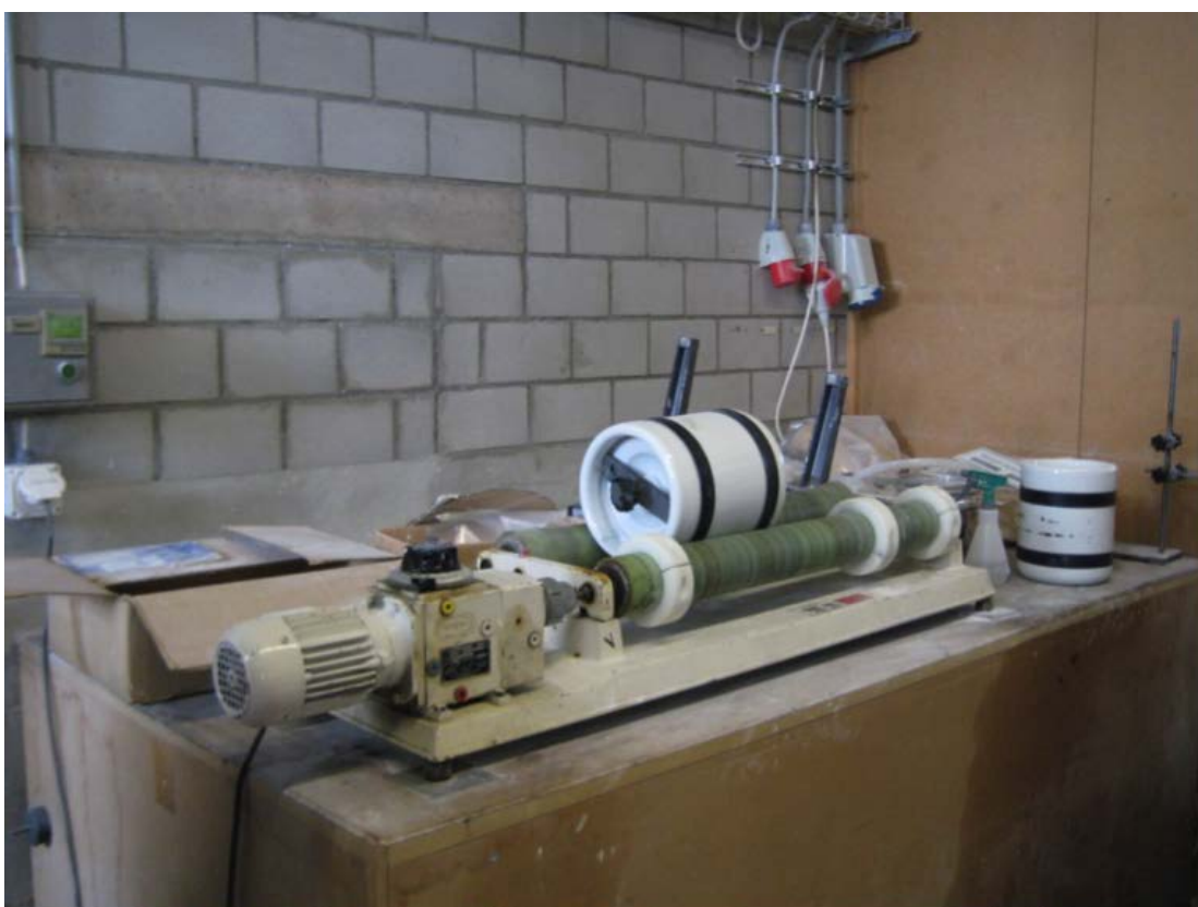
Figure 4.4: A ceramic cylinder, inside of which contains the sample centrifuge tubes, was placed on two rollers powered by a motor (Alpine Augsburg 1/25 LK) in order to continuously agitate the samples.
