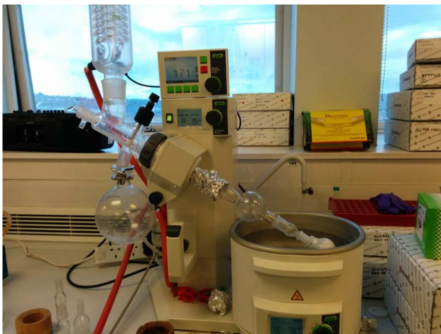
Figure 5.2: A round-bottomed flask with saccharin, FCC, and ultrapure water undergoing rotary evaporation.
