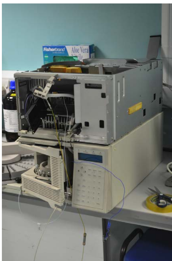
(c) A photograph of the DAD module of the HPLC when dismantled in order to gain an appropriate angle to drill through the bolt.
