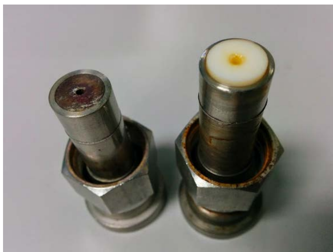
Figure 3.10: A photograph of the brass and PTFE inserts used in ZLC liquid designs.
