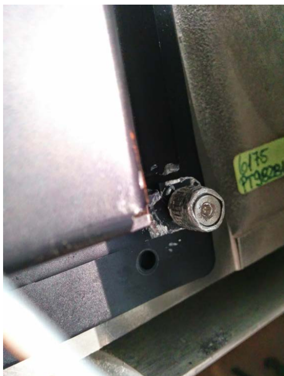
(a) A photograph of the bolt sealing the flow cell assembly inside the black box.
