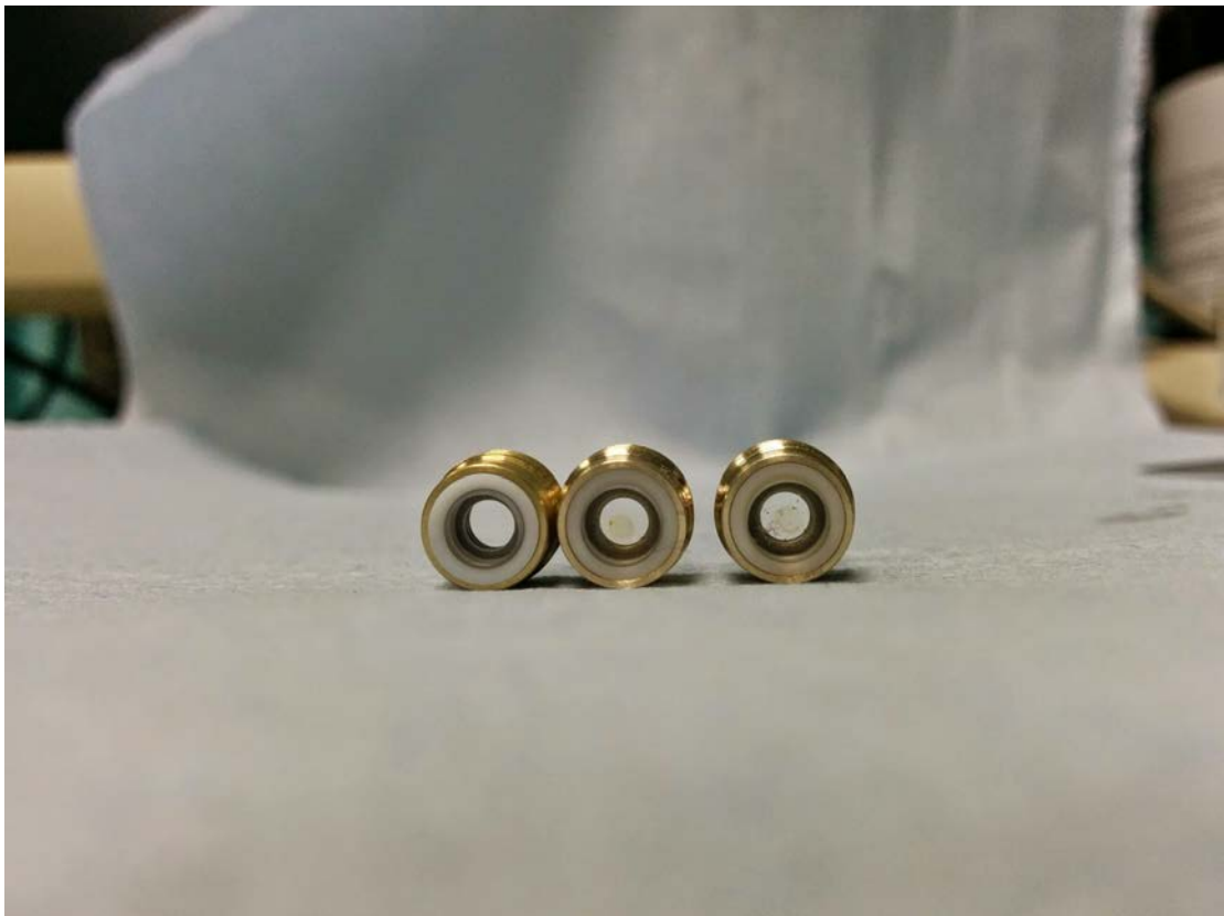
(c) A photograph of flow cell window cartridges; the leftmost cartridge is new and clean while the middle and rightmost cartridges were the ones being replaced in the HPLC. It is apparent that the cartridges taken from the HPLC are visibly dirty when compared to the new cartridge.
