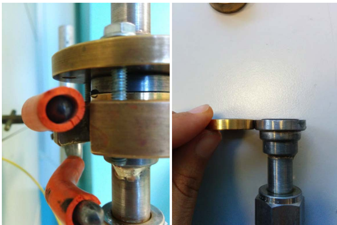
(a) A photograph of the FLC leaking during an experiment.
