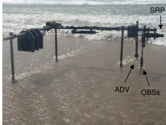
Fig. 3. Instrumented rig in-situ , showing the Sand Ripple Profiler (SRP), Acoustic Doppler Velocimeter (ADV) and Optical Backscatter Sensors (OBSs). The cylinders to the side contain the batteries, conditioning electronics and data loggers.
