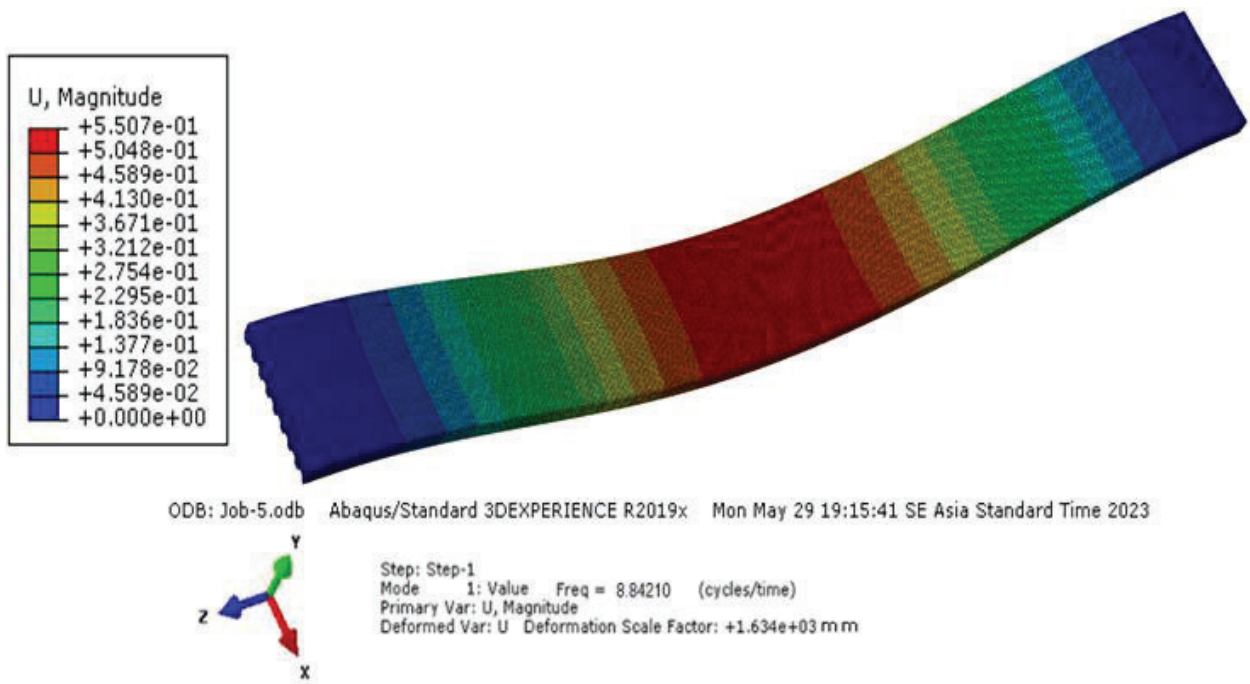
Fig. C3. Mode shape Frequency response of slab RCA100% slab for Model 3
