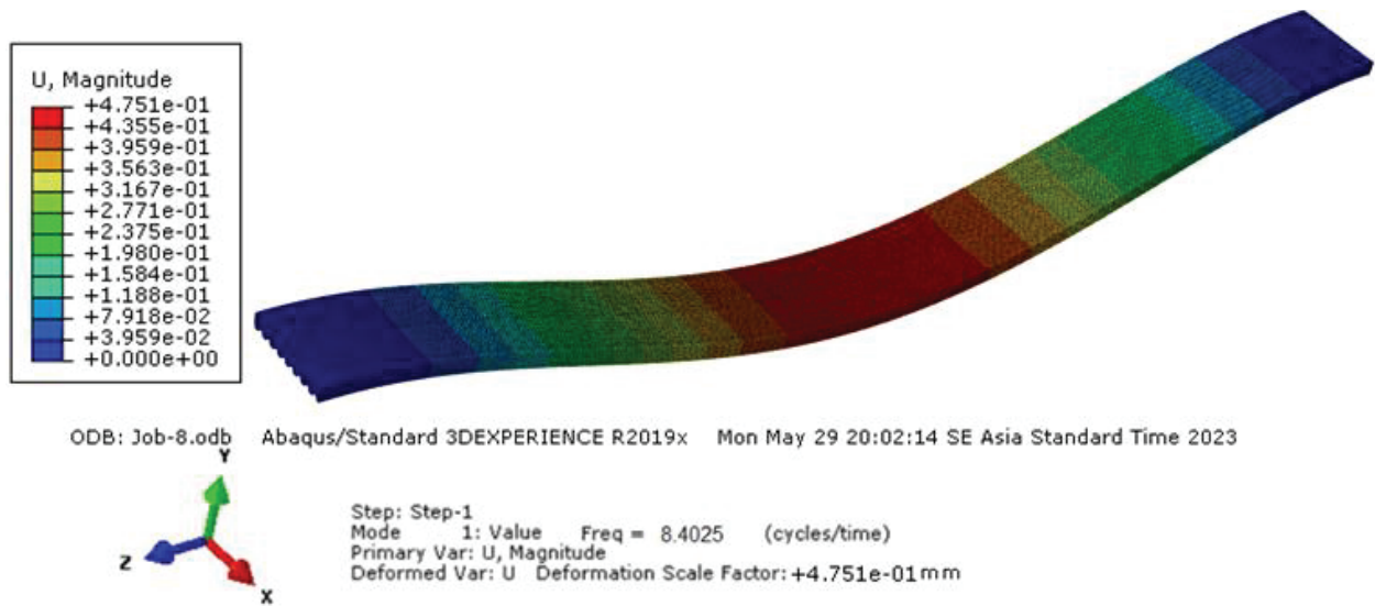
Fig. C5. Mode shape Frequency response of slab RCA100% slab for Model 5
