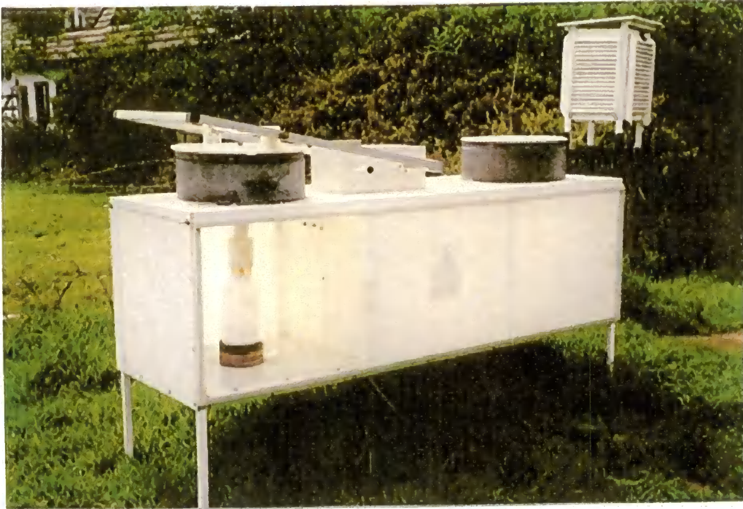
Plate 3.1: the wet/dry deposition collector at the western English Channel sampling site.
