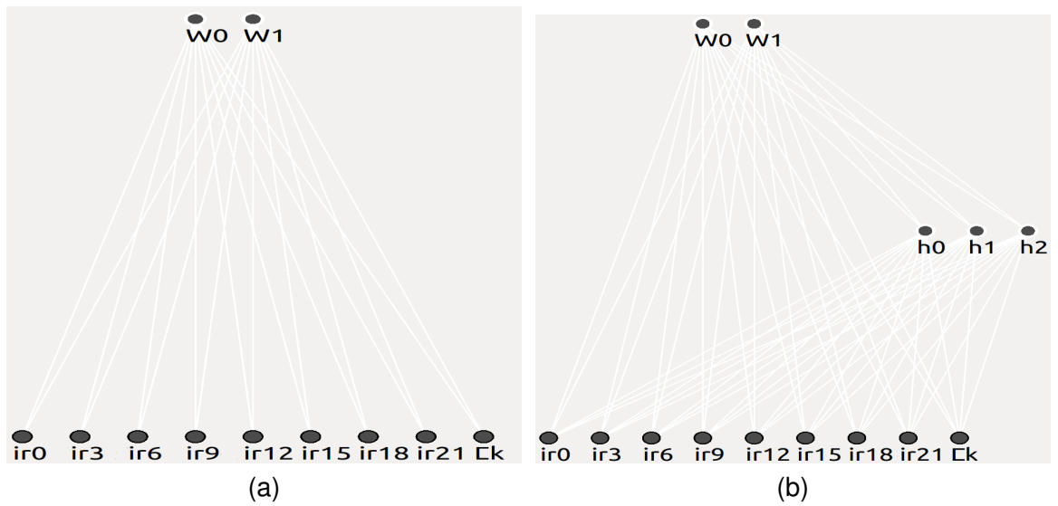
Figure 3.4: Time Neural Network Controller with (b) and without (a) hidden neurons. The output neurons W define the motor activation for left and right wheels of the robot. Neurons with a white contour around it mean the presence of a bias parameter. The input Ck is the internal clock that varies linearly from 1 to 0 along the trial.
