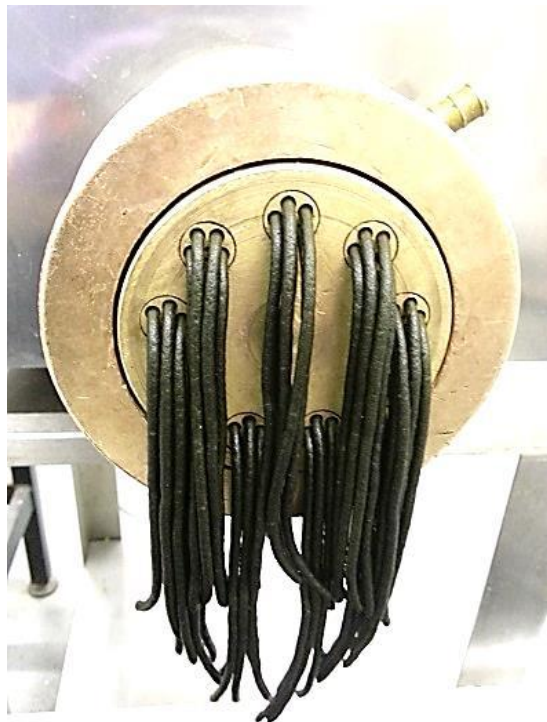
Figure 2.2 Extrusion of 2mm strands of formulated diet through brass die prior to drying.
