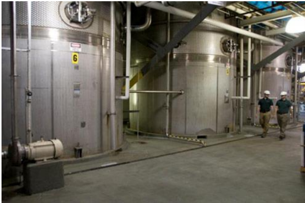
Figure 1.8 Modified brewery fermentation towers used for heterotrophic algae biomass production, some of the largest in the world – Kentucky, USA.
