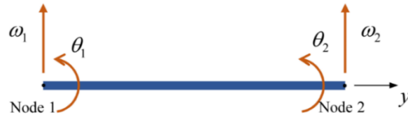
Fig.5 Beam element in local coordinate system
