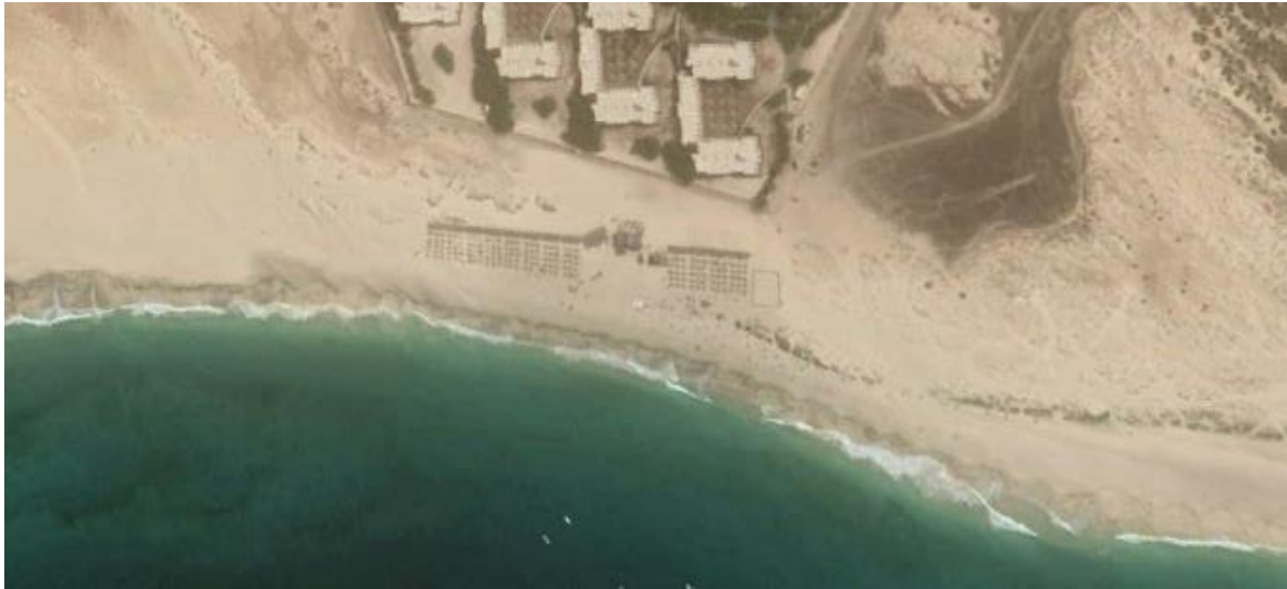
Figure 2-3. Aerial imagery of Riu Funana beach showing beach cusp formations at the shoreline.
