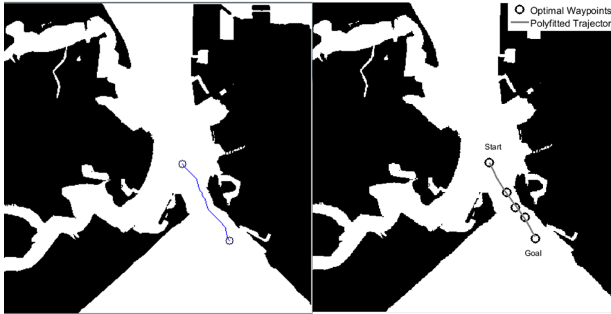
Figure 10. Generated (left) and smoothed trajectory (right) from the optimal waypoints produced by the path planner. Binary map of 800 \times 800 resolution is considered for the current study with one pixel representing 3.6 m on a real map.
