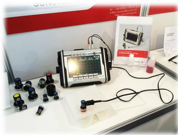
Fig. 4.24. SONOTEC SONOSCREEN ST10, a compact ultrasonic flaw detector, together with several transducers for use in NDT of plastics and composites, demonstrating structural defect on the surface of a plastic structure.
