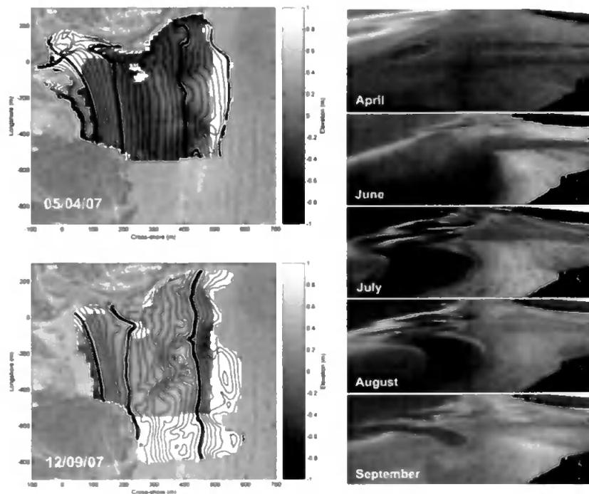
Figure 6. (left) 3D RTK GPS surveys at Perranporth shown as residual elevations from a mean surface at the start and end of the 2007 spring/summer season and (right) monthly spring low tide Argus TIMEX images give overview of observed changes during the 2007 spring/summer study period.
