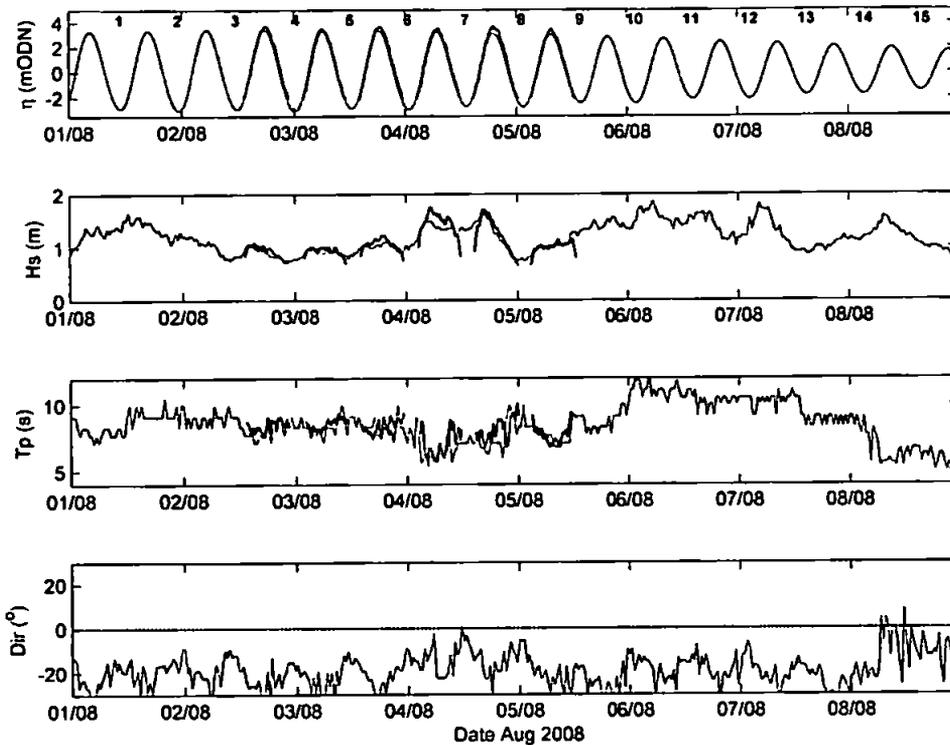
**Figure 6.6** – (Top) Tidal elevation record from a UoP prediction model (grey) and the TWR (black); (below) Wave record from the DWR (grey) and TWR (black), showed measured values for significant wave height ( $H_s$ ,  $T_p$ ) and wave direction relative to shore normal. The DWR is located  $\sim 1$  km from the shore in 10 m water depth.
