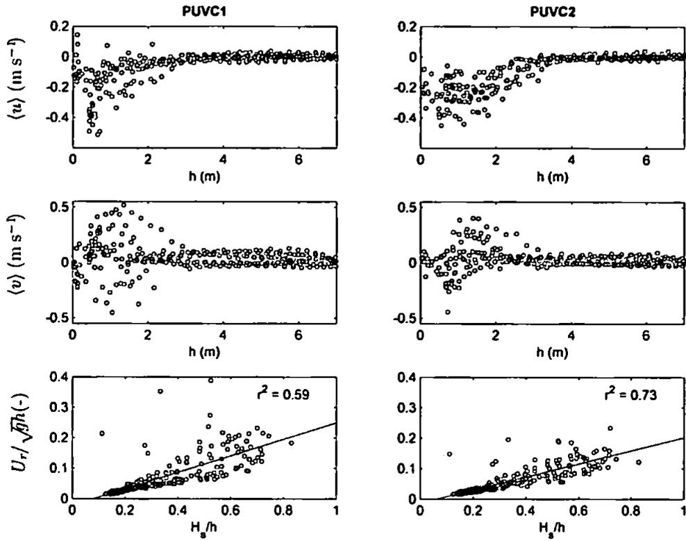
**Figure 6.11** - Scatter plots of (top) mean cross-shore current and (middle) mean longshore current vs. water depth; and (bottom) Froude number vs. relative wave height on the bar crest indicating linear fit.
