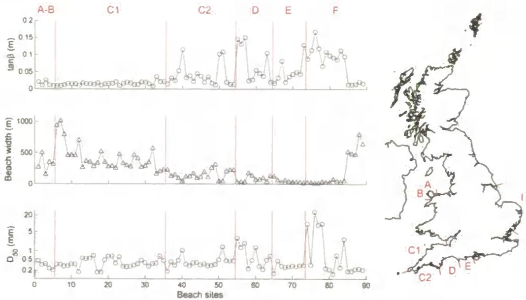
**Figure 4.12** – Summary profile morphometrics and sediment size for all beach sites moving anti-clockwise around the coast: (top) mean spring inter-tidal beach slope; (middle) mean spring inter-tidal beach width; and (bottom)  $D_{50}$  for the lower inter-tidal zone at each beach site.
