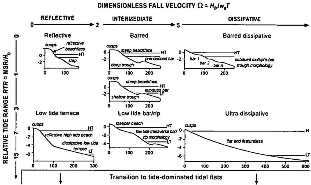
Figure 1.16. - Modified conceptual beach state model (Masselink and Short, 1993).
