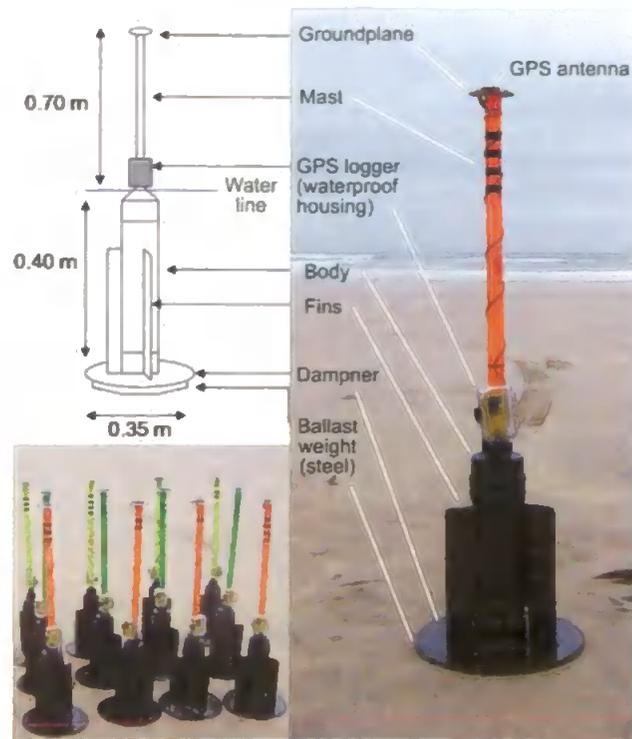
**Figure 6.4** – Picture (right – not to scale) and diagram (upper left) of the inexpensive surf zone drifter that the GPS was deployed on. The main body buoyancy is built of upvc tube and welded end caps on top of a round, flat, plywood (marine) disk to dampen and prevent surfing. Below this a steel plate acts as ballast. The design is based on that of (MacMahan et al., 2009b; Schmidt et al., 2005).
