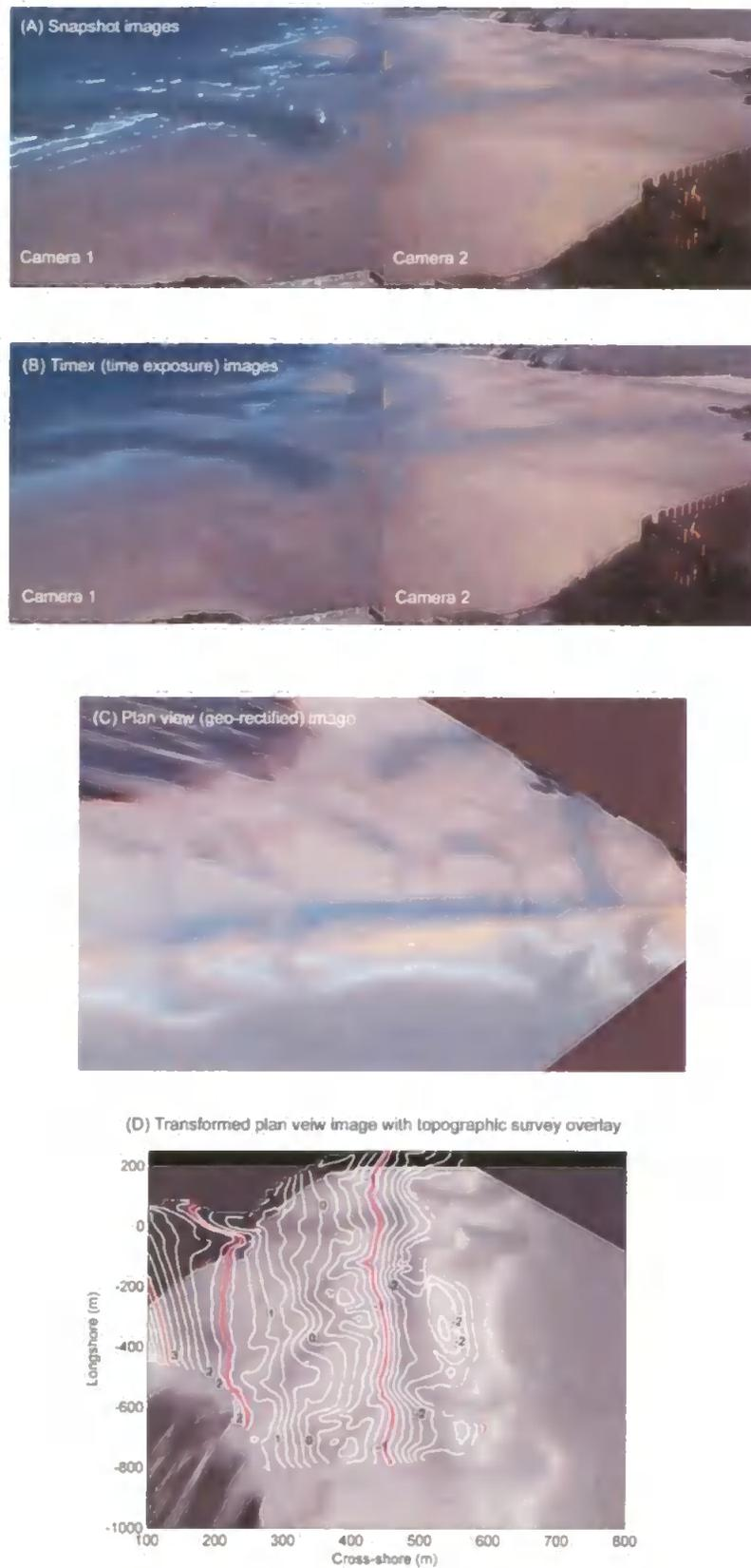
**Figure 2.7** - Example Argus video products from Perranporth station: (A) snapshot images; (B) timex images; (C) plan view (geo-rectified) image; and (D) example of low-tide plan image transformed into local co-ordinates for merge with survey data.
