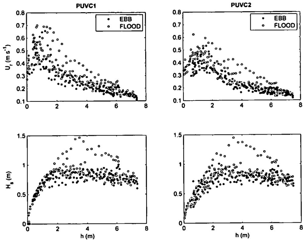
**Figure 6.10** – Return flow velocities  $U_r$  during the flood and ebb tides (top) for feeder and rip rigs (PUVC 1 and 2 respectively). (Bottom) Comparison of observed significant wave height  $H_s$  during the flood and ebb tides. Data are observations from entire deployment.
