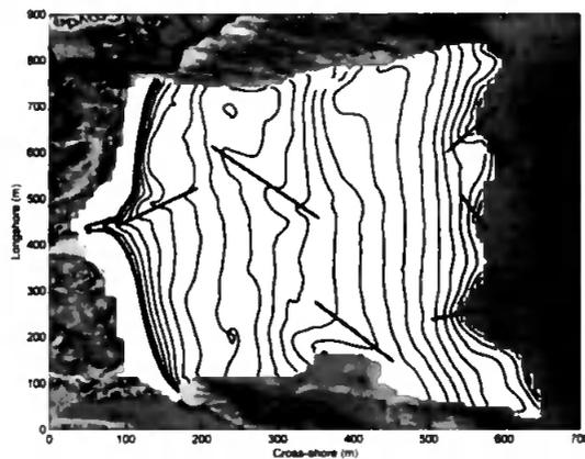
**Figure 10. Plots A and B show 15 minute shorelines at Croyde Bay, North Devon during spring tides on the 18/06/07 and 14/09/07 respectively. Bold grey lines indicate regions of heightened rip current hazard.**
