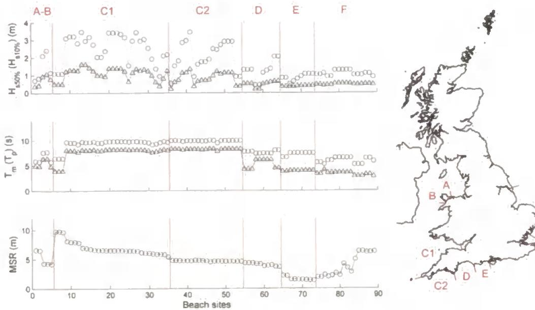
**Figure 4.11** – Nearshore hydrodynamic conditions for each beach site moving anti-clockwise around the coast: (top) 50% exceedence significant wave height (triangles) and 10% exceedence significant wave height (circles); (middle) mean wave period (triangles) and peak wave period (circles); and (bottom) mean spring tidal range.
