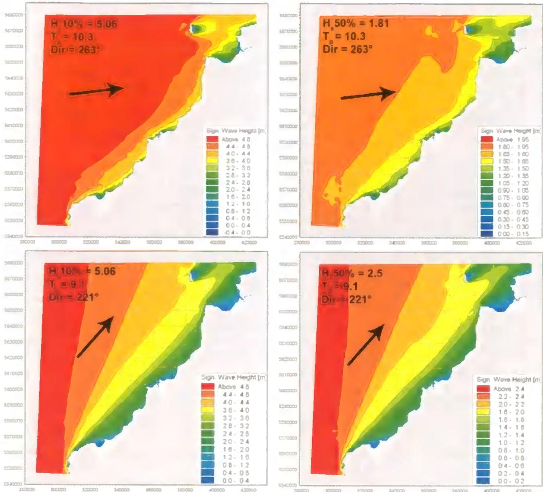
**Figure 2.17** – Example of four model runs for the Atlantic west coast representing the  $H_{s,10\%}$  and  $H_{s,50\%}$  exceedance levels (left to right) for both west and southwest swell directions (top to bottom).
