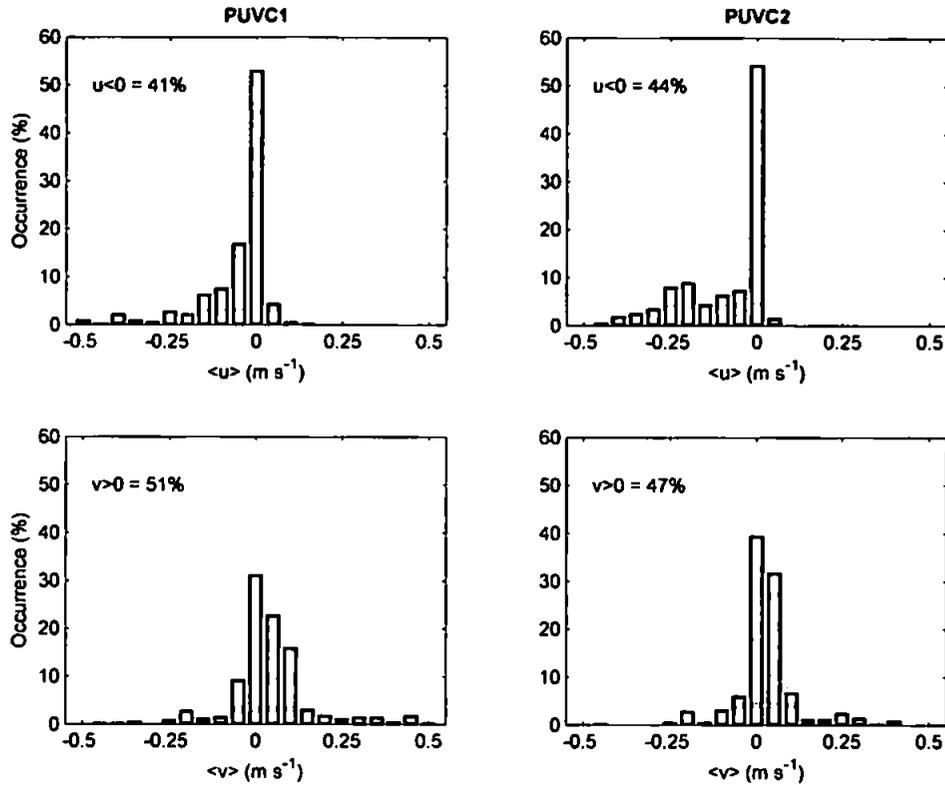
**Figure 6.9** – Histograms of 8.5 min mean velocities of; (top) cross-shore, onshore directed; and (bottom) longshore, northward flows from the rip (PUVC1) and feeder (PUVC2) instrument locations. Measurements represent observations from LT(3, 4, 5, 7 and 8).
