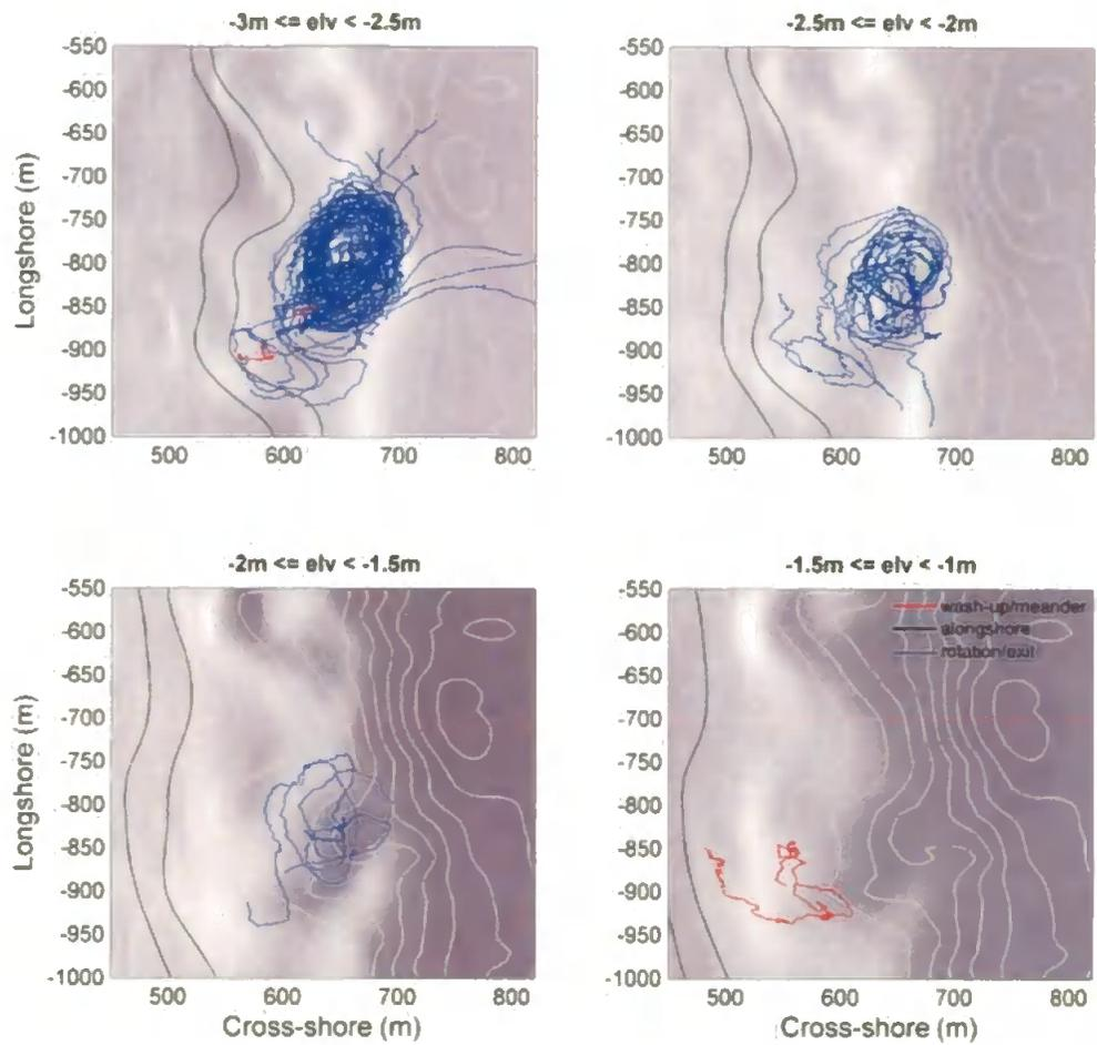
**Figure 6.19** – Drifter tracks for LT5 (03/08/08), separated into 0.5 m sea-surface elevation bins. Colours represent associated behavioral classification. Background rectified video image represents nearest capture to the bin midpoint.
