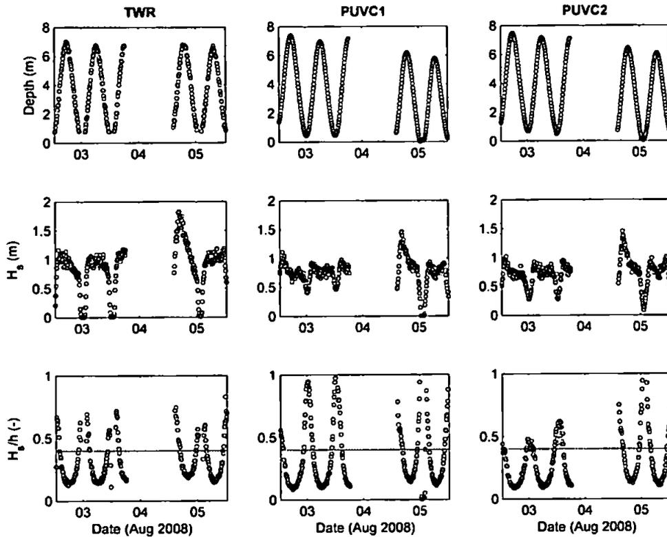
**Figure 6.7** – Summary of statistics of measured sea surface elevation from the in-situ instruments at 10 minute intervals. (Top) Mean water depth above the instrument position. (Middle) Significant wave height,  $H_s$ . (Bottom) A measure of relative local relative wave height,  $H_s/h$ . The dashed line on bottom panel at  $H_s/h > 0.4$  indicates approximately value for the onset of wave breaking (Thornton and Guza, 1982).
