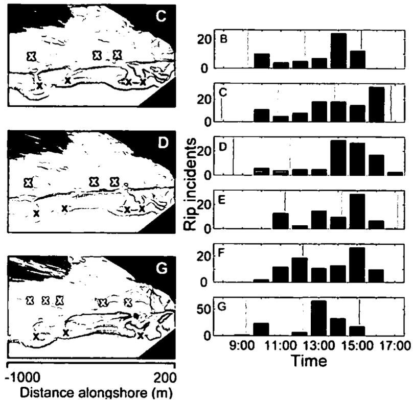
**Figure 5.27** – (Left) Time averaged, rectified, low-tide video images of Perranporth during events C, D and G; sea is located at the bottom of each image, land at the top. West is oriented down-page; black markers locate approximate positions of low-tide rip currents, white locates mid-tide rip channel morphology. (Right) Histograms of incident times for each event from all beaches. Dark shading indicates 3 hour low-tide period and light shading the mid-tide.
