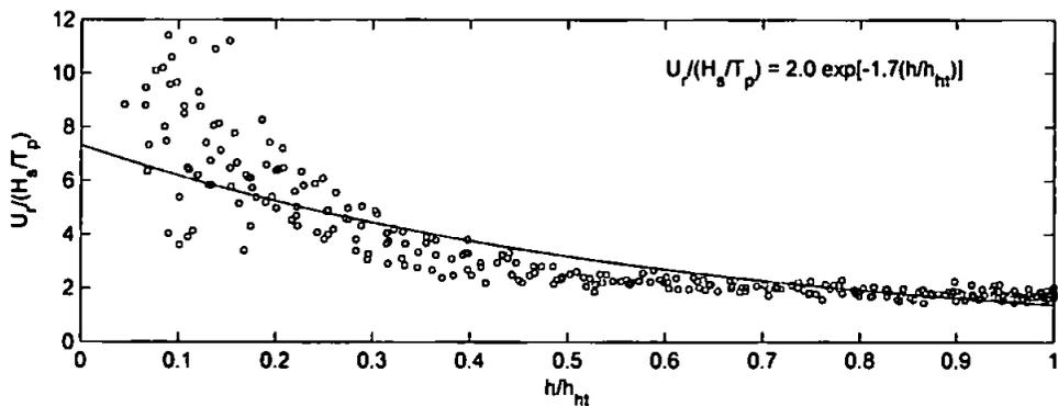
**Figure 6.12** – Plot illustrating the relationship between mean rip return flow, non-dimensionalised by wave steepness  $(H_s/T_p)$ . Curve represents the exponential relationship of rip velocity scaling from Brander and Short (2001).
