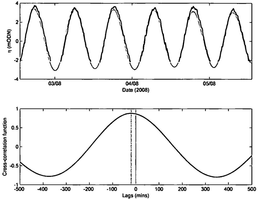
**Figure 6.17** – Comparison of predicted and measured sea-surface elevation. (Top) predicted tide (grey) and measured surface elevation,  $\eta$  (black). A consistent lag on the falling limb of the tide can be seen in the TWR data. Lag is also observed on the rising limb to a lesser extent. (Bottom) The cross-correlation function of the time series in the upper panel indicating a negative lag of 20 mins (dotted line).
