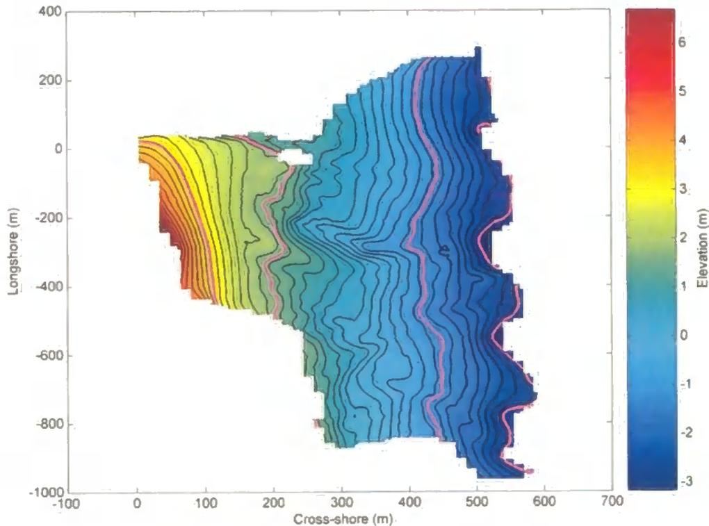
**Figure 2.5** - Typical resultant interpolated surface DEM from Perranporth using quadratic loess interpolation routine. Interpolation scales ( $\lambda_x$ ) = [5; 10; 30; 50] m; Grid spacing ( $x$ ) = 5 m; and permissible vertical interpolation error levels set at 0.05 m. Magenta lines indicate mean tidal levels. Black lines are contoured elevation at 0.25 m intervals.
