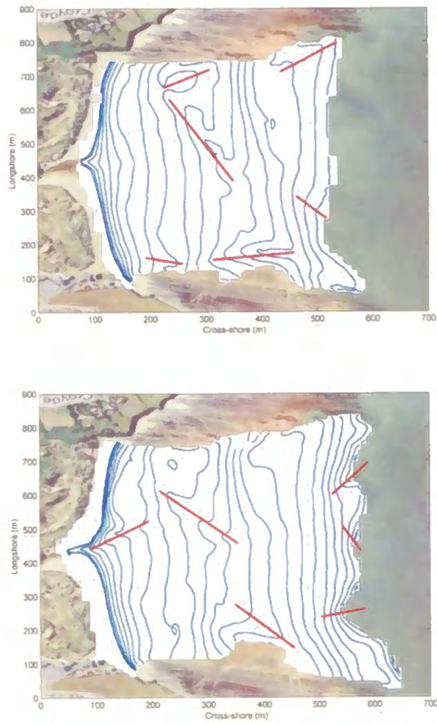
**Figure 5.28** – Plots A and B show 15 minute shorelines at Croyde Bay, North Devon during spring tides on the 18/06/07 and 14/09/07 respectively. Bold red lines indicate regions of heightened rip current hazard.
