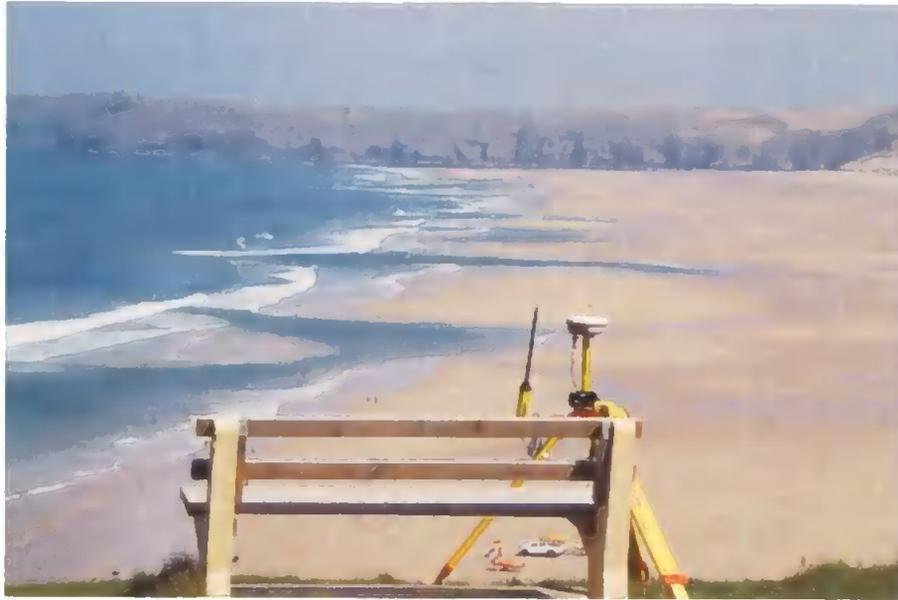
**Figure 2.1** - Reference base station for the RTK GPS survey system. Trimble 5800 dual frequency receiver and radio with battery pack (12Ah). Perranporth beach in the background provides a good example of typical low-tide morphology in the region.
