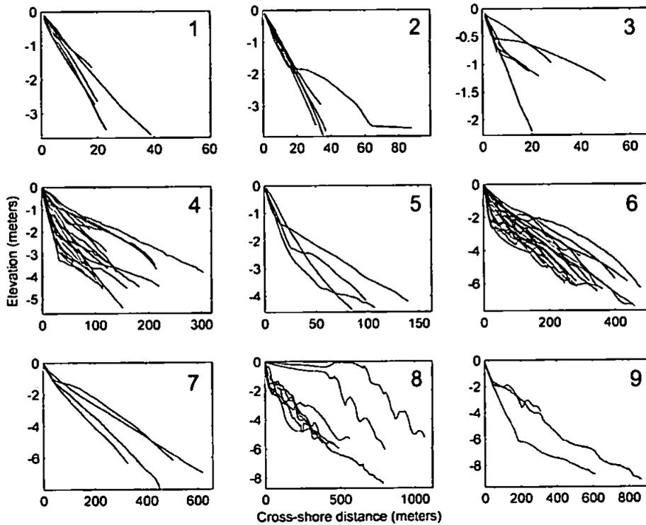
**Figure 4.19** – Cross-shore profiles of beach sites within each morphotype grouping: (above) fixed scale indicates relative cross-shore and vertical extents; (below) scale to fit plots show individual profile geometries. Numbers indicate beach group.
