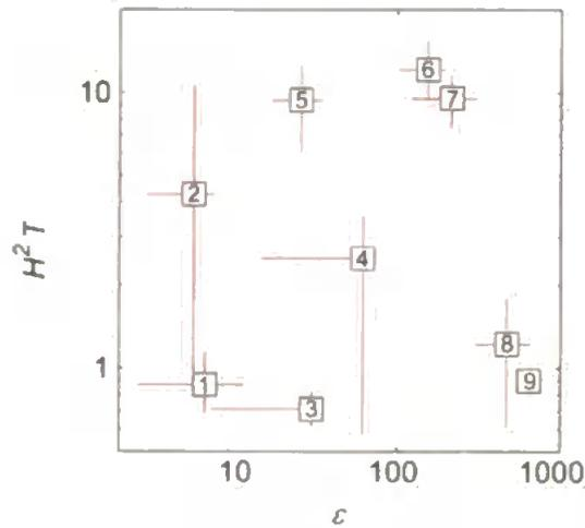
**Figure 4.24** – Plot of deep water wave energy flux scaling parameter ( $H_{50\%}^2 \cdot T_m$ ) against the surf scaling parameter. Boxes indicate modal values for each group and stems are values of the 25th and 75th percentiles of the group distribution.
