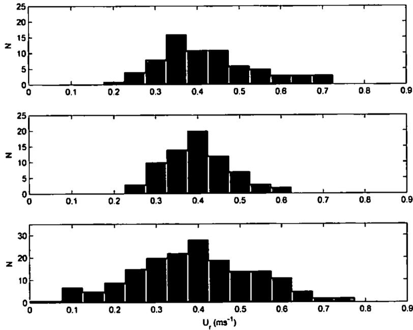
**Figure 6.15** - Comparison of Eulerian and Lagrangian drifter speeds  $U_r$ . Mean rip current speeds at PUVC1 (top) and PUVC2 (middle) during periods when the rip current was active ( $\eta < -1$  mODN). (Bottom) Rip speed from the statistically significant mean drifter circulation during periods when drifter and in-situ instruments were synchronous.
