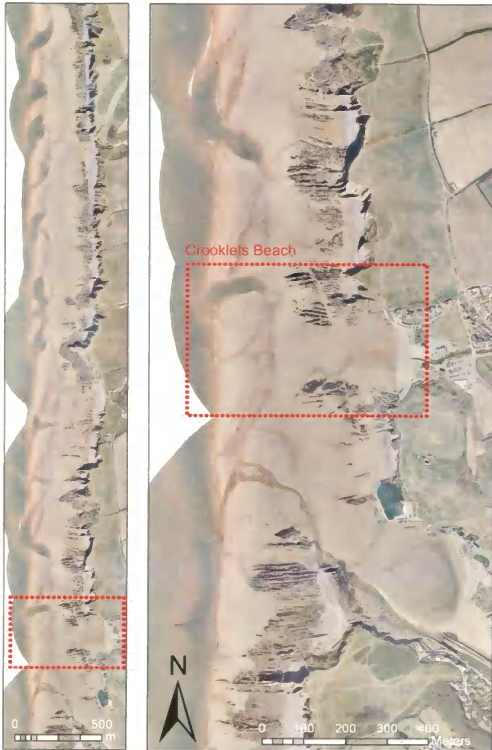
**Figure 5.19** – Aerial images of Crooklets beach (September 2006) and associated constrained upper inter-tidal morphology and open lower inter-tidal bar systems. Images provided by the Environment Agency.
