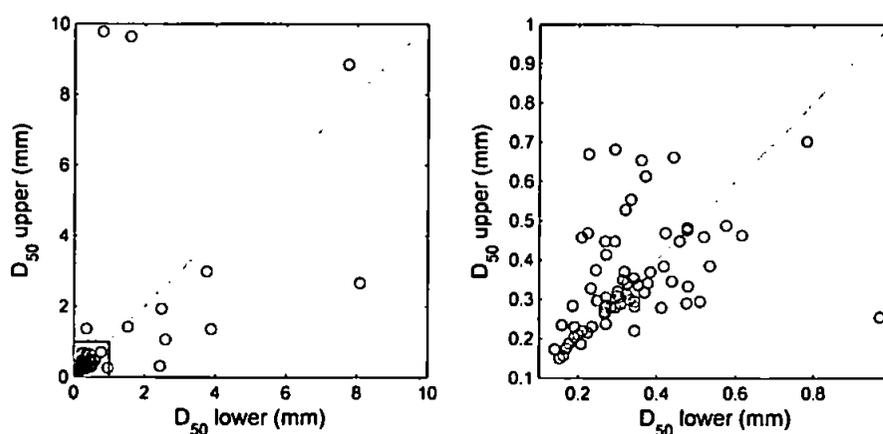
**Figure 4.14** – Plots showing relationship between upper and lower  $D_{50}$  at all beach site (excluding Orford Ness where  $D_{50}$  upper = 26.32 mm and  $D_{50}$  lower = 21.05 mm): (left) all samples < 10 mm with exploded plot marked; (right) exploded view of all samples < 1 mm.
