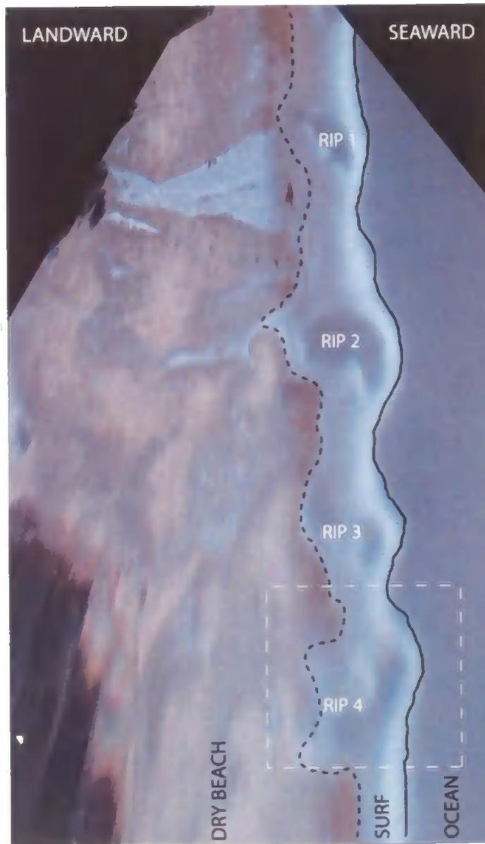
**Figure 6.1** – Rectified low tide ARGUS image of rip currents at Perranporth during experiment period. The dashed and solid black lines represent the shoreline position and the seaward edge of the surf zone. The four rips are separated by transverse bars and retained within the surf zone by a longshore bar (sinuous bright band demarcating outer surf zone). The boxed area represents experiment region.
