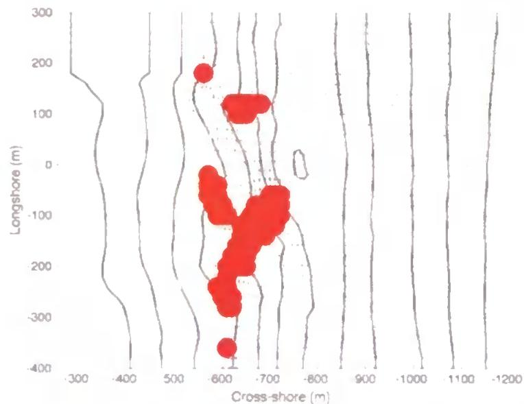
**Figure 7.3** - Example of Rip Risk Plot showing the occurrence of offshore-directed mean nearshore currents exceeding 0.5 m/s. The plot was obtained using XBeach with standard parameters (uncalibrated) and the measured bathymetry (not derived from using the BeachWizard).
