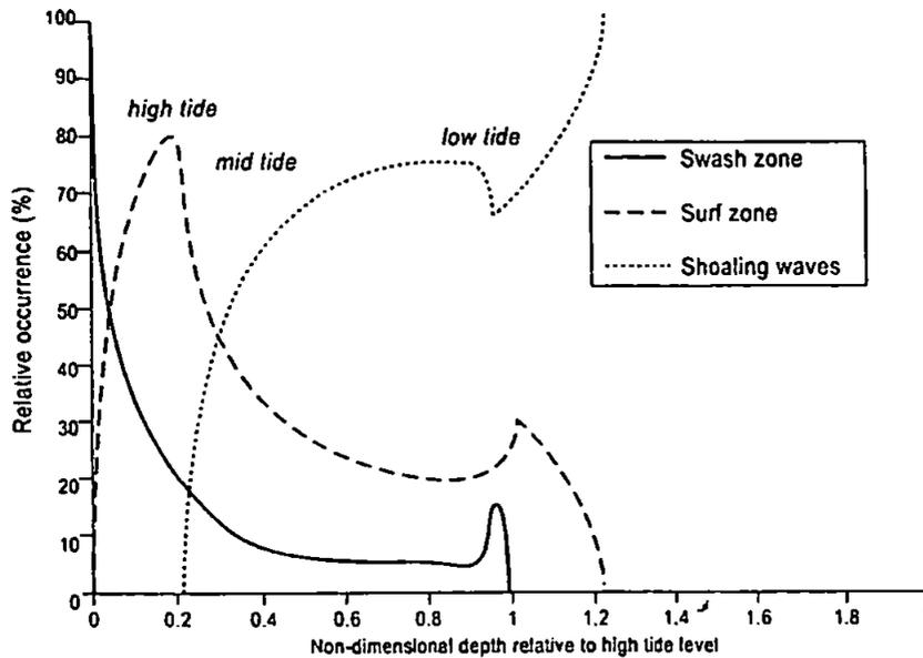
**Figure 1.15.** - Relative occurrence of swash, surf and shoaling wave processes across the beach profile calculated over one tidal cycle where  $H = 1$  m,  $T = 8$  s,  $w_r = 0.03$  m s<sup>-1</sup>, breaker criterion  $\gamma = 0.8$  and tide range  $TR = 6$  m from a simulated tidal excursion model by Masselink and Short (1993).
