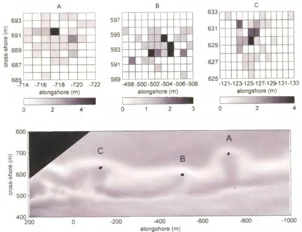
**Figure 2.9** - Sensitivity analysis of observational consistency during manual rip picking routine. Top three panels show picked rip head locations for 150 acquired points. The three rip locations are indicated on the Argus plan timex image in bottom panel.
