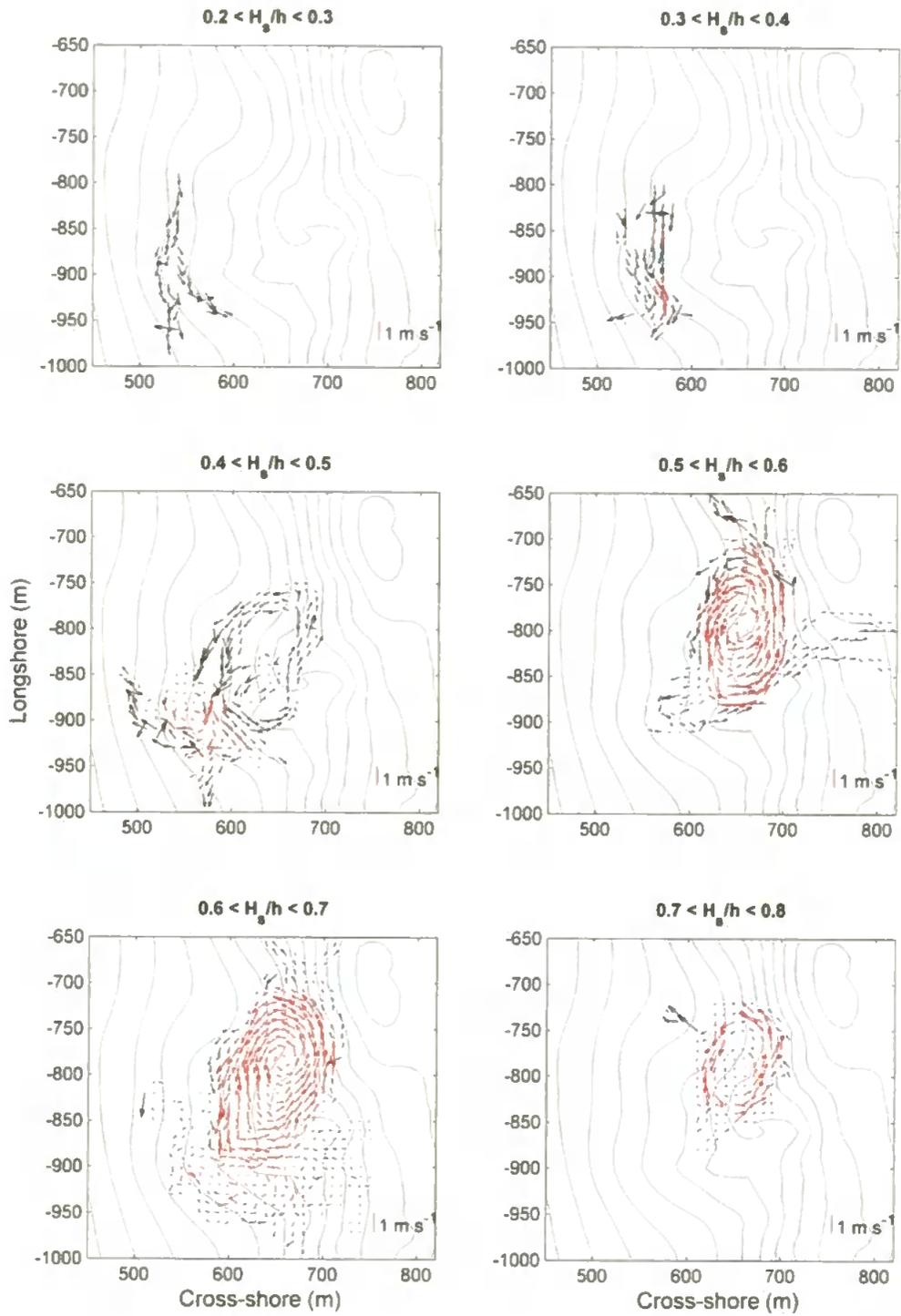
**Figure 6.24** – Observed mean Lagrangian rip circulation associated with each  $H_b/h$  bin (width 0.5). Red vectors represent significant velocities ( $> 5$  independent observations). Colours indicate mean return speeds associated with each  $10 \text{ m} \times 10 \text{ m}$  bin. Bathymetry is contoured in background.
