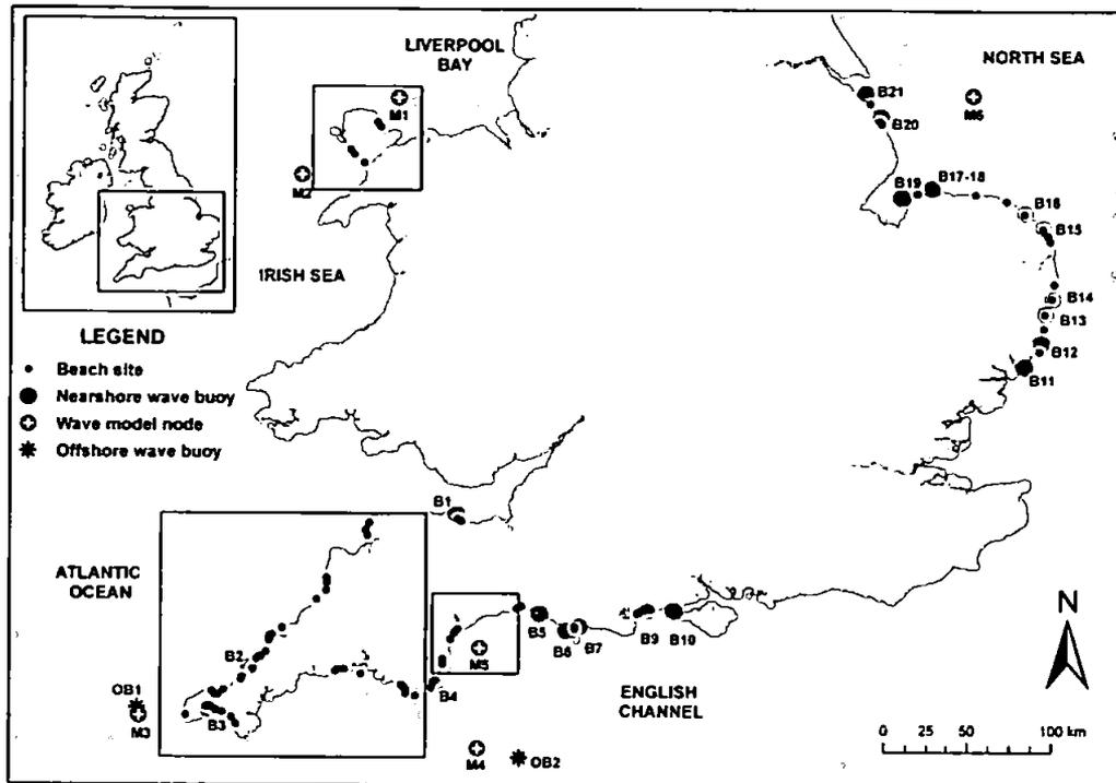
**Figure 2.12** - Overview map of wave data sources used in the study. UK beach study sites are marked by black filled circles. Boxes indicate regions where nearshore wave modelling was performed using MIKE21.
