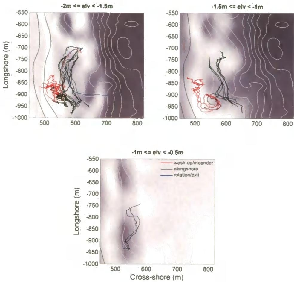
**Figure 6.22** – Drifter tracks for LT13 (07/08/08), separated into 0.5 m sea-surface elevation bins. Colours represent associated behavioral classification. Background rectified video image represents nearest capture to the bin midpoint.
