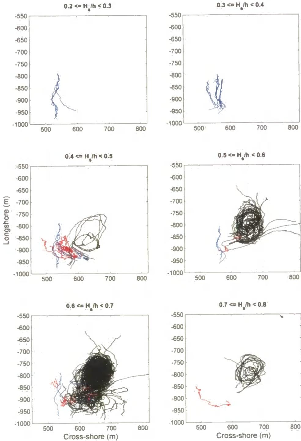
**Figure 6.23** – Combined drifter tracks from LT3, LT5 and LT7, separated into  $H_s/h$  bins of 0.5. Colours represent associated behavioural classification: rotation (black); alongshore (blue); and wash-up/meander (red). Measured bathymetry represented in background.
