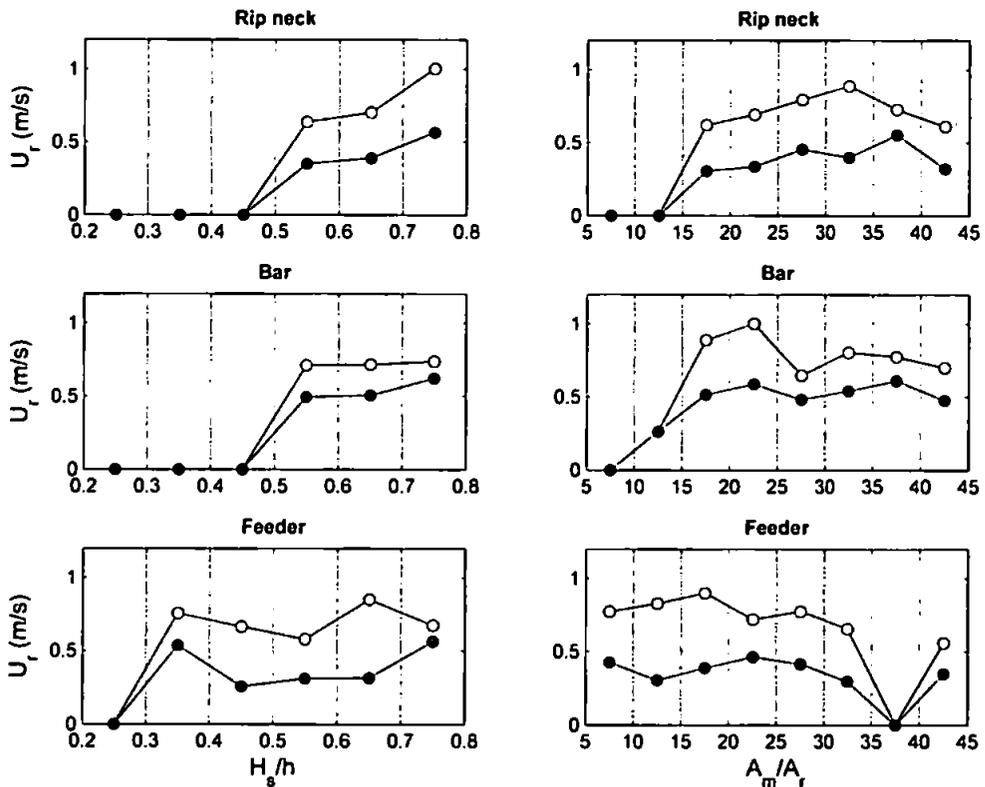
**Figure 6.28** – Mean and maximum rip speeds  $U_r$  associated with rip neck (offshore-directed), bar (onshore-directed) and feeder regions. Values are separated into  $H_s/h$  (left) and  $A_m/A_r$  (right) classes. Dashed lines indicate class boundaries.
