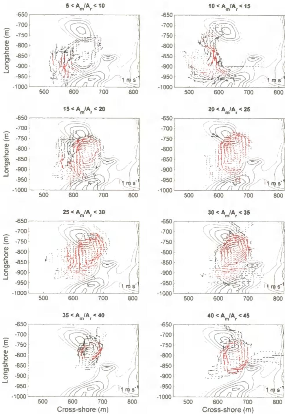
**Figure 6.26** – Mean Lagrangian rip circulation separated into  $A_m/A_r$  classes. Shading indicates mean rip speed  $U_r$  within each spatial bin for all observations. Vectors (red) represent rip speed for those bins classified as statistically significant ( $> 5$  independent observations). Residual bathymetry is contoured in the background.
