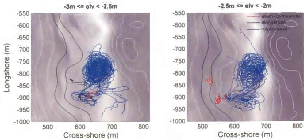
**Figure 6.20** – Drifter tracks for LT7 (04/08/08), separated into 0.5 m sea-surface elevation bins. Colours represent associated behavioral classification. Background rectified video image represents nearest capture to the bin midpoint.
