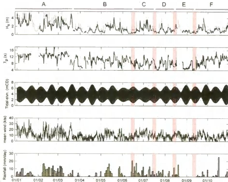
**Figure 5.11** – (from the top) Offshore wave record (6 hour averaged) during study period ( $H_s$  and  $T_p$ ) Grey line shows simultaneous 6 hr averaged offshore wave record from Seven Stones Lighthouse; predicted tidal elevation (mCD); mean hourly wind speed and daily rainfall totals from St Mawgan airfield. Red regions highlight survey periods.
