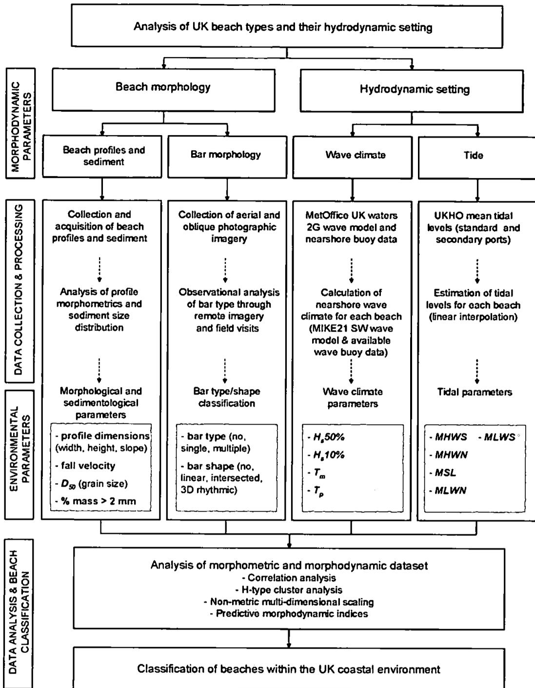
Figure 4.3 – Flow diagram of research methodology for this beach classification study.
