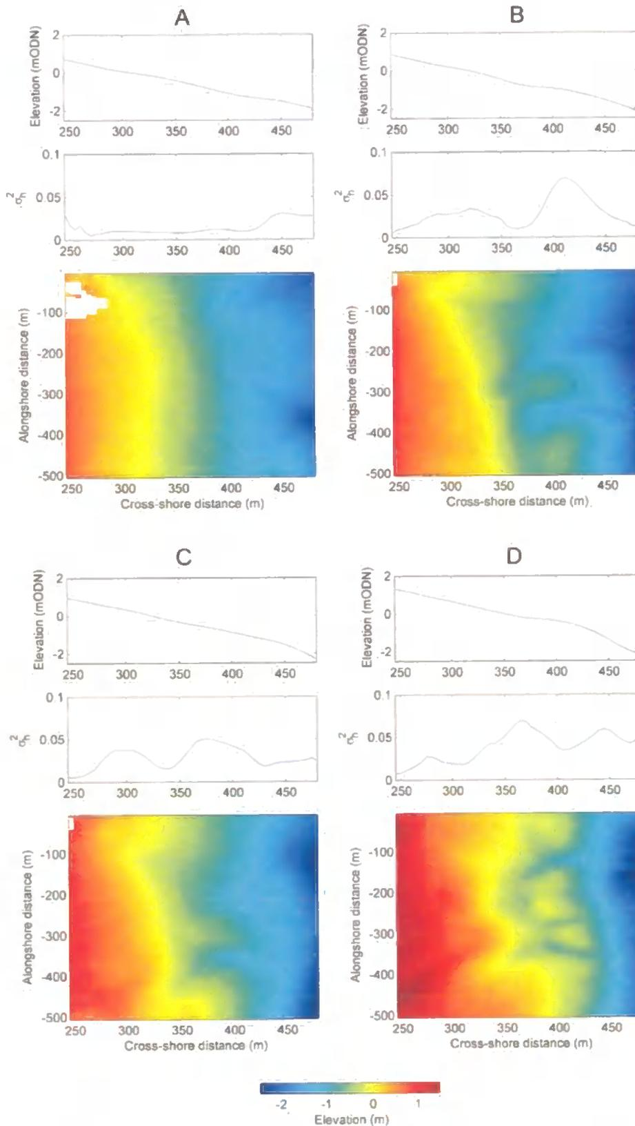
**Figure 5.13** – Panels A-D show, for selected region; (from top) alongshore averaged cross-shore profile; cross-shore variation in bathymetric non-uniformity ( $\sigma_b^2$ ); and three-dimensional surface elevation for Perranporth beach. A – 05/04/07; B – 18/07/07; C – 15/08/07; and D – 12/09/07.
