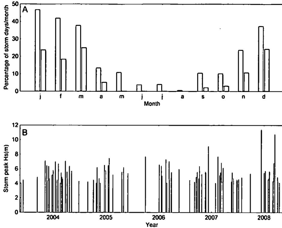
**Figure 1.8** – Temporal characteristic of storm events in the southwest of England (Seven Stones offshore wave buoy, 2003 – 2008). Storm duration defined as the time over which the mean hourly  $H_s$  remained above 2 m: (A) storm days per month, grey and white bars represent storm peak  $> 4$  m and  $> 6$  m, respectively; (B) Peak wave heights ( $H_s$ ) for storms identified between 2003 and 2008.
