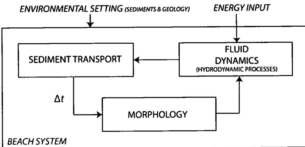
**Figure 1.10.** – Primary components involved in beach morphodynamics. The feedback loop is responsible for the fundamental complexities in beach morphological evolution.  $\Delta t$  represents the time dependence inherent in morphological evolution due to the process of sediment redistribution.
