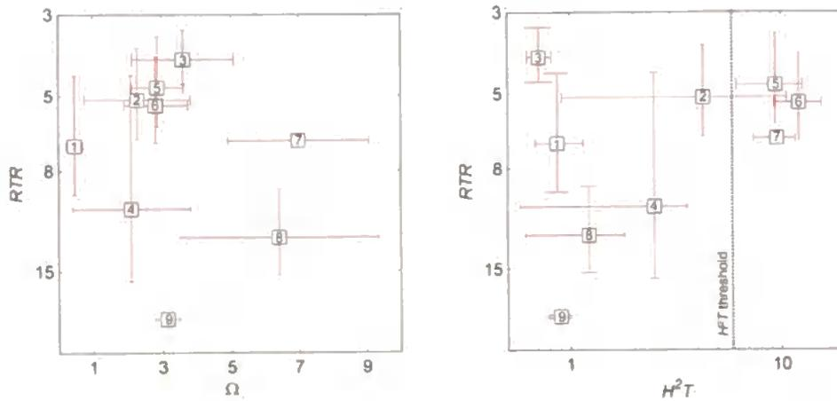
**Figure 4.26** – Plot of  $\Omega$  (upper beach) against  $RTR$  (left) and deep water wave energy flux ( $H_{s50\%}^2 \cdot T_m$ ) against  $RTR$  (right). Boxes indicate modal values for each group and stems are values of the 25th and 75th percentiles of the group distribution. Numbers indicate beach group.
