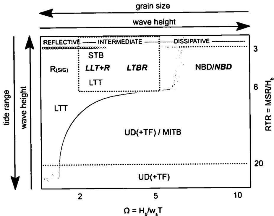
**Figure 4.28** – Conceptual morphodynamic framework for sampled UK beaches. Dark and light shading indicate transition from reflective to dissipative surf zone conditions respectively. Black dashed box indicates region where high-energy conditions ( $H^2T > 5 \text{ m}^2 \text{ s}$ ) induce 3D bar formations and bold italics represent high-energy beach types.
