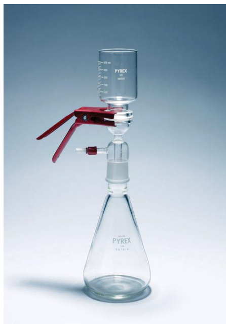
Figure 26) Filtration system used for separation of suspended material (Source: SciLabWare Ltd)
