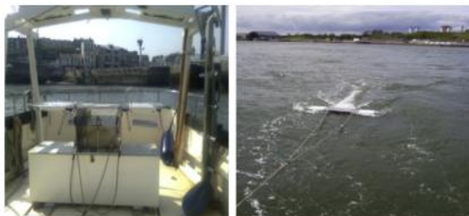
Fig. 2. Manta net on board RV Aquatay (left) and deployed in the Tamar Estuary (right). The overall width of manta including its floating wings was ~150 cm.
