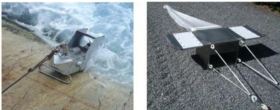
Figure 25) Photographs of the Continuous Plankton Recorder (left) and Manta net (right).
