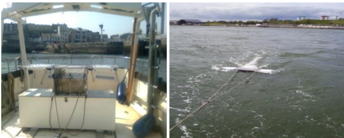
Figure 35) Manta net on board RV Aquatay (left) and deployed in the Tamar Estuary (right). The overall width of manta including its floating wings was ~ 150cm.
