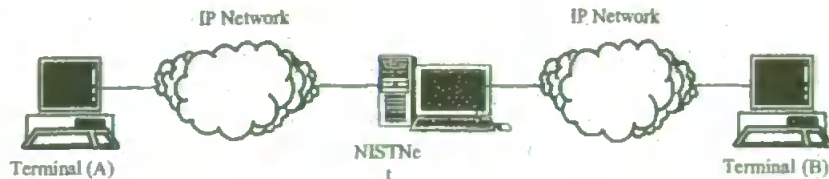
Figure 1: Test Bed Configuration
