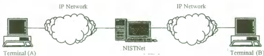
Figure 1: Test Bed Configuration
