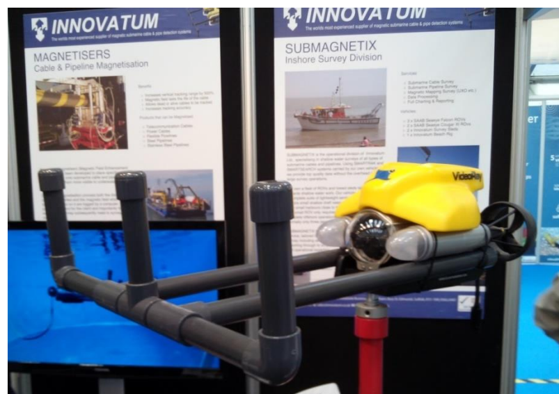
Figure 30 Innovatum sensor array mounted on small ROV and displayed during Marine Expo
