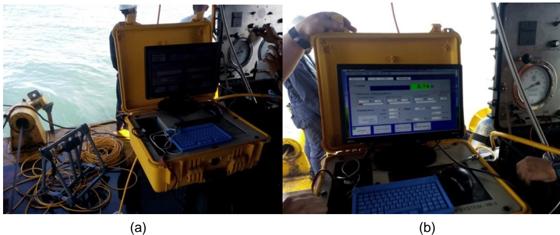
Figure 29 (a): equipment preparation for diver inspection during cable burial in South America 2015. (b): Burial depth confirmation by a diver
