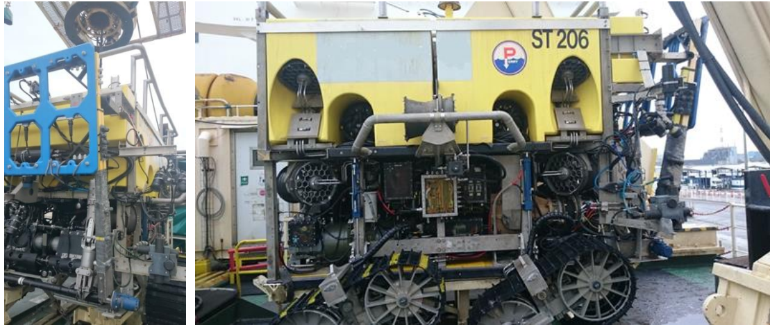
Figure 26 The TSS system mounted on the ROV used by one of the cable layer ship (courtesy Subsea Cable Tracking Ltd)
