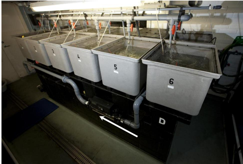
Plate 2.1 Recirculation system 'D' located at Plymouth University. White arrow shows the direction of water over flow to experimental tanks from the drum filter through the biological filter (not visible).
