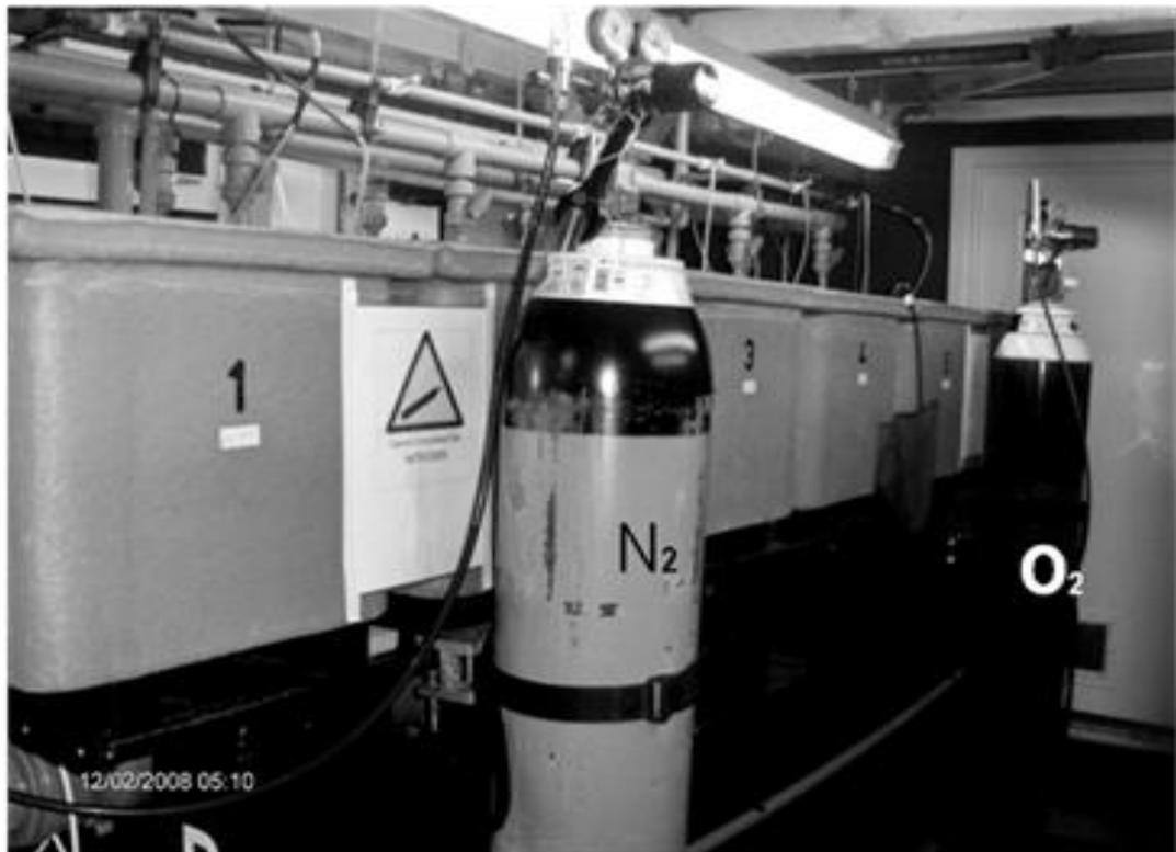
Plate 4.1 A view of the experimental set up using nitrogen and oxygen cylinders to maintain hypoxia and hyperoxia in the water tanks.
