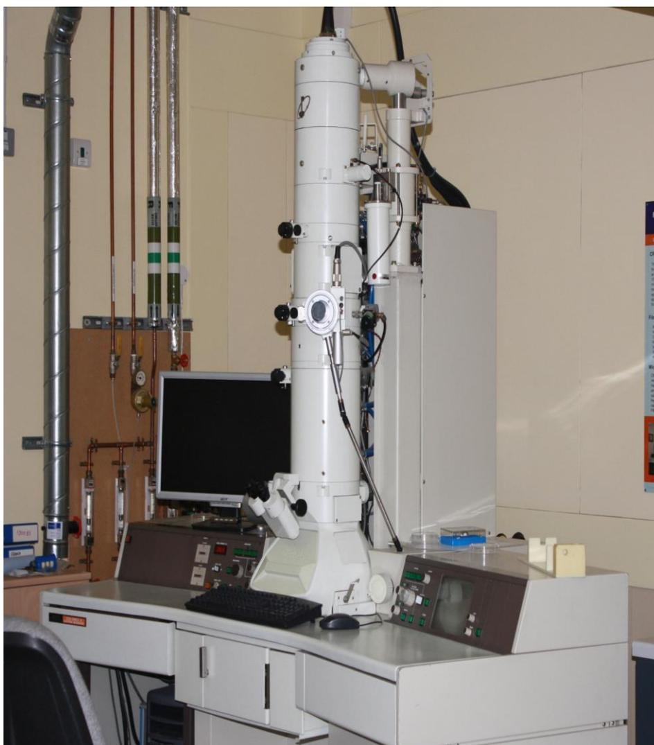
Plate 2.6 JEOL, TEM-1200EX II used for TEM analysis.
