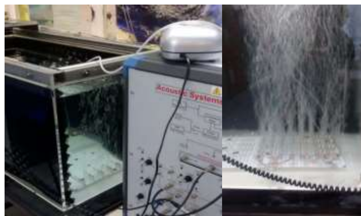
Figure 4.2: Bubble screen generation apparatus. Left: An air pump connects to a single air-line affixed to the bottom of the tank producing a single bubble screen. Right: Eight bubble screens in series at 3 cm separation.
