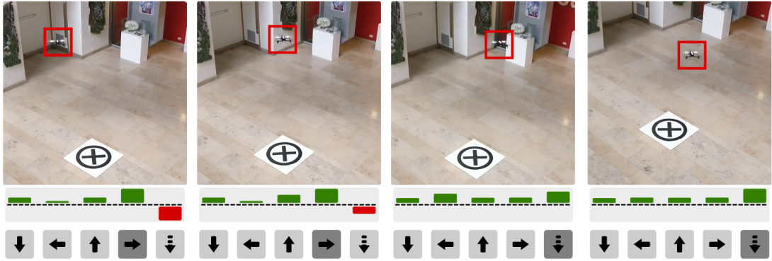
Figure 5.17: Snapshots representing vertical descent in the large hall environment. The bottom bar is the utility distribution of the actions. Descent has a negative utility (red bar) when the UAV is not centred on the marker.
