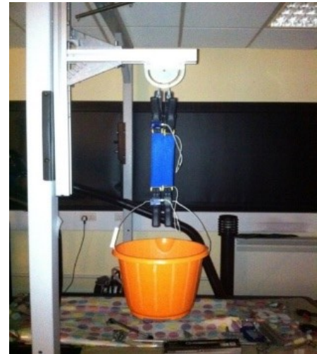
Figure 2.1 Apparatus laboratory set up for fabric stiffness testing
