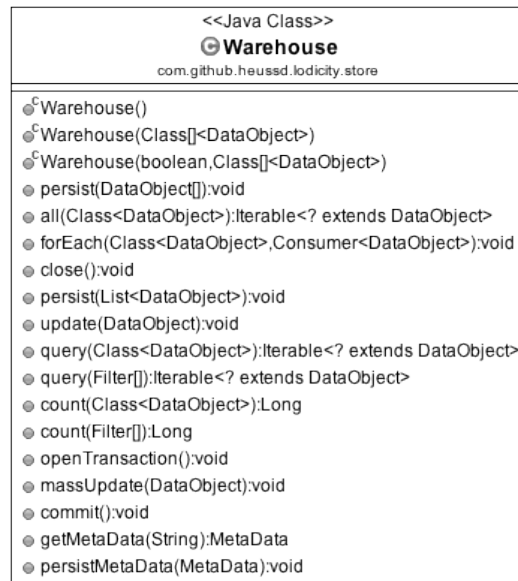
Figure 4.22: UML Class Diagram of Warehouse.
