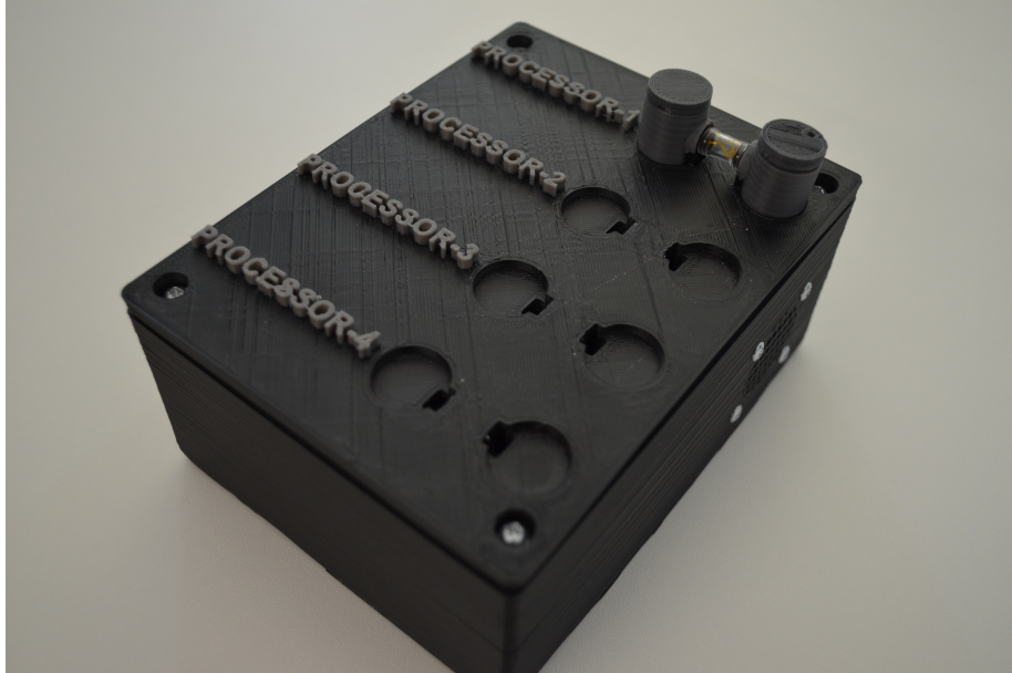
Figure 4.3: PhyBox. A micro-kernel to use Physarum polycephalum -based memristors as processing units.
