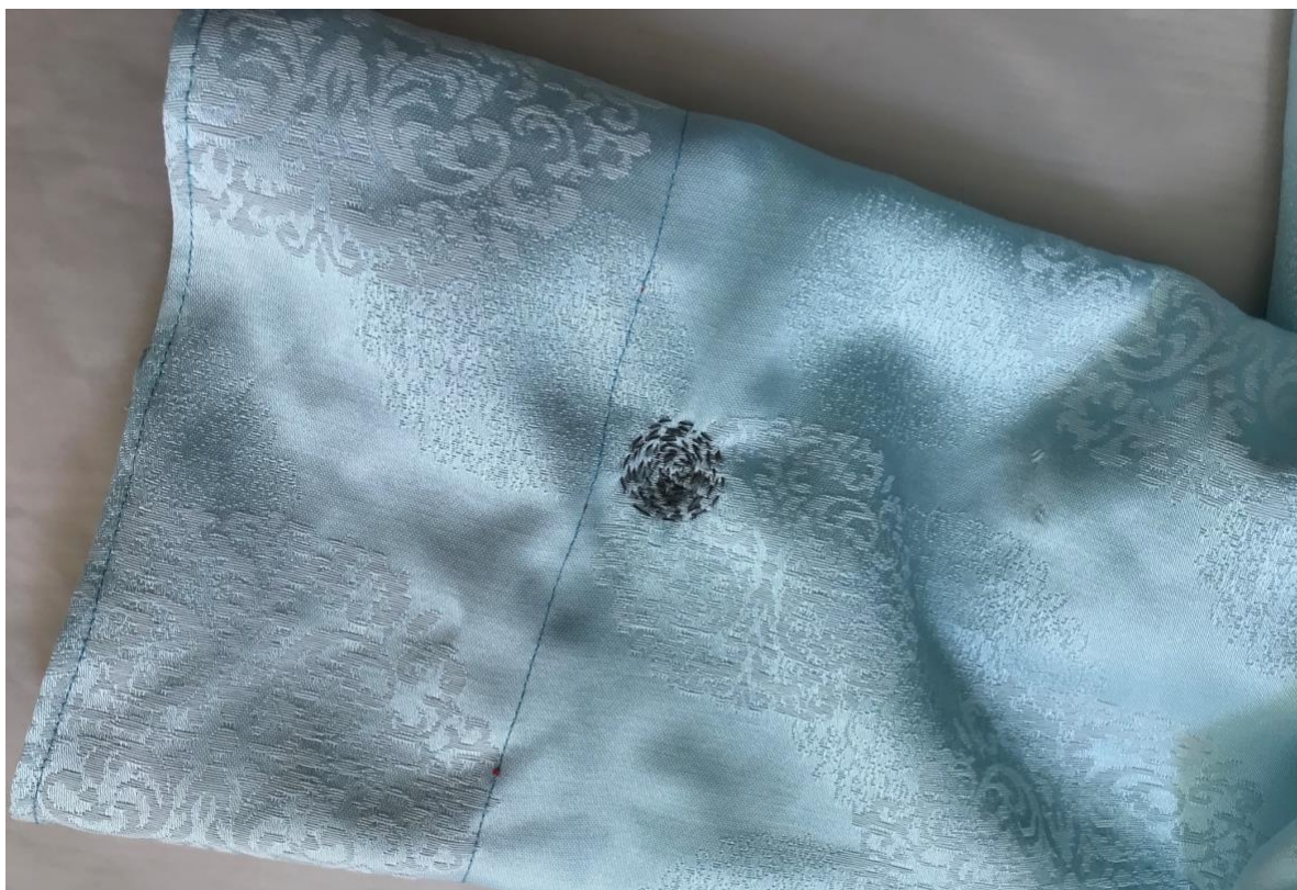
Figure 21: Detail of final version of dress sleeve and embroidered conductive thread button.
