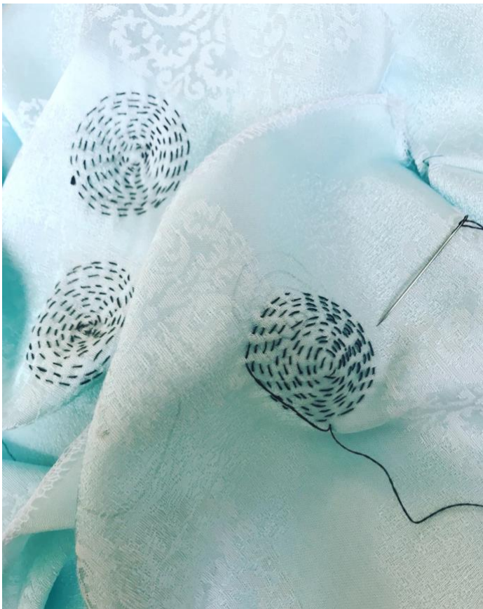
Figure 29: Detail of conductive thread hand sewn buttons in circular patterns.
