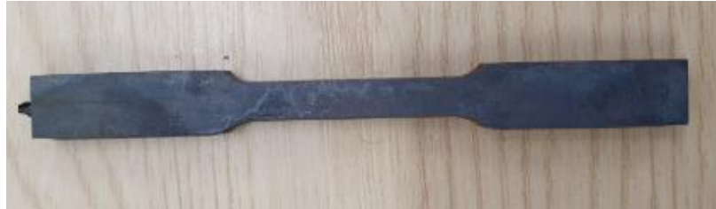
Figure 2: Tensile test specimen after manufacturing.
