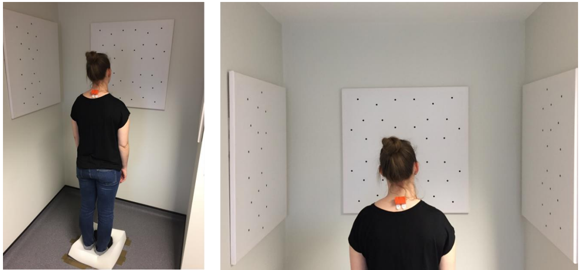
Figure 7.3: Postural sway set up with pilot participant standing on foam surface condition with eyes open and central + peripheral visual scene. Xsens accelerometer is attached to skin, overlying T1 vertebral spinous process, with two latex-free double sided, self-adhesive strips.
