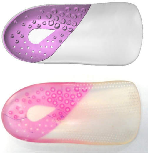
Figure 6.3 First CAD/CAM model produced from CT scan (top) of the prototype orthosis (bottom) (Simpleware, 2010)
