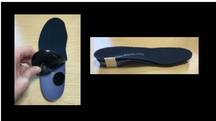
Figure 7.2 Positioning and blinding of the discs on the Vectorthotic™ shell
