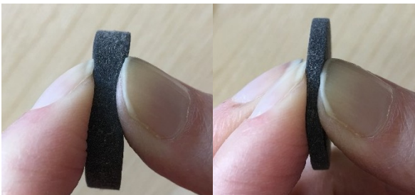
Figure 6.7 Prototype two in 3 mm and 6 mm thick versions
