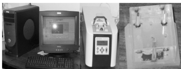
Fig. 1 MDK™ Power supply and micro reactor; electrodes were fabricated within the base plate of the micro reactor.
