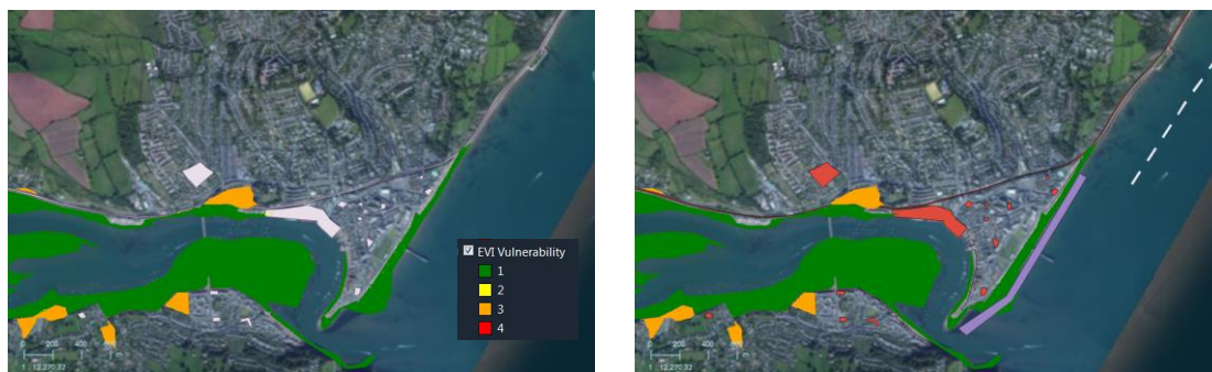
Figure 7. EVI vulnerability: No mitigation options (up) vs All mitigations (down). Mid-term conditions: 2050 yr, Tr 50 yrs. Scale: Low (green), Moderate (yellow), Medium (orange) and High (red) risk.
