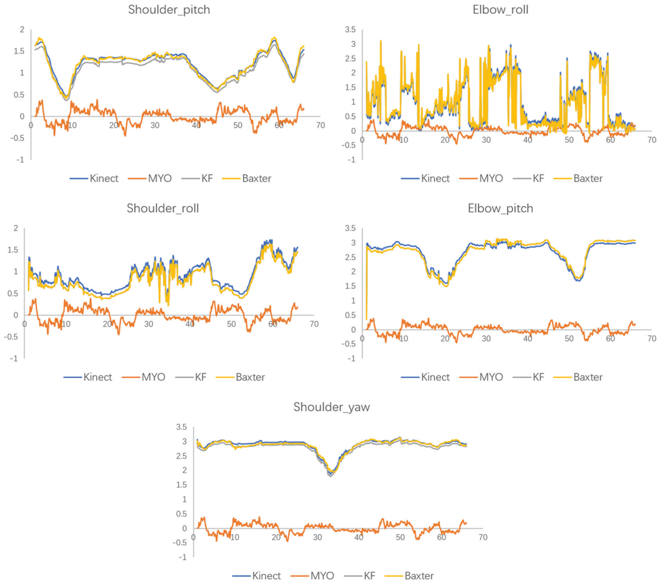
Figure 13. Graphical result after the Kalman Filter-based sensor fusion ( Shoulder Pitch, Shoulder Roll, Shoulder Yaw, Elbow Pitch, Elbow Roll).
