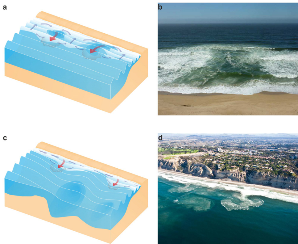
Fig. 9. Examples of bathymetrically-controlled rip currents: (a) schematic of channel rip currents flowing offshore over a rip head bar or through an incised channel between sand bars with predominant shore-normal wave approach; (b) channel rip current at Marina Beach, California (photo Rob Brander); (c) schematic of focused rip currents showing offshore bathymetric hole; (d) focused rip currents (sediment plumes) at Blacks Beach, California (photo Tom Cozad).
