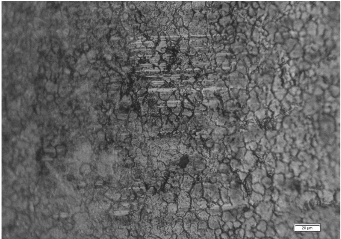
Figure 4-26 DoE 001a x50 Abrasive wear due to the substrate imperfections
