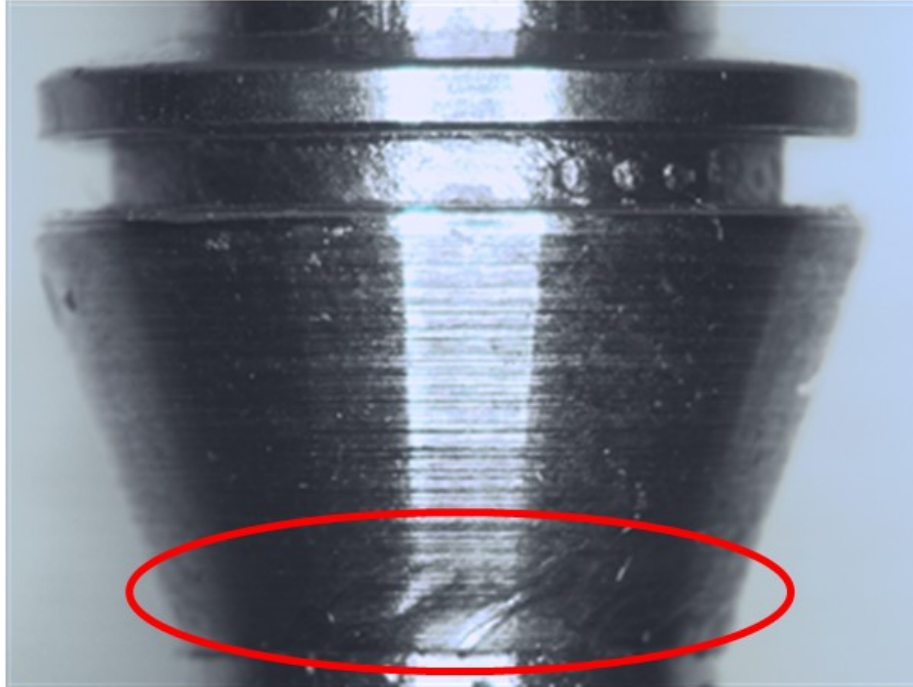
Figure 6-8 Galling damage on front ferrule observed from the fifth attempt of non-cyanide Ag coating
