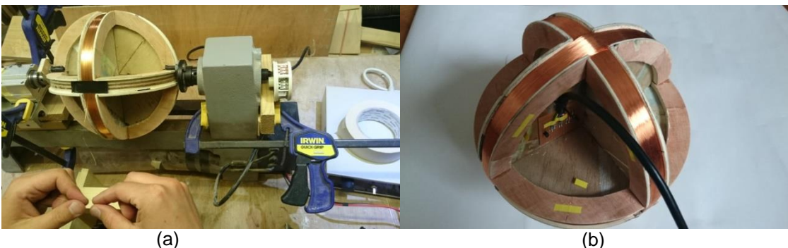
Figure 34 Air coil with a diameter of 200 mm; (a): coils during production; (b): final sensor
