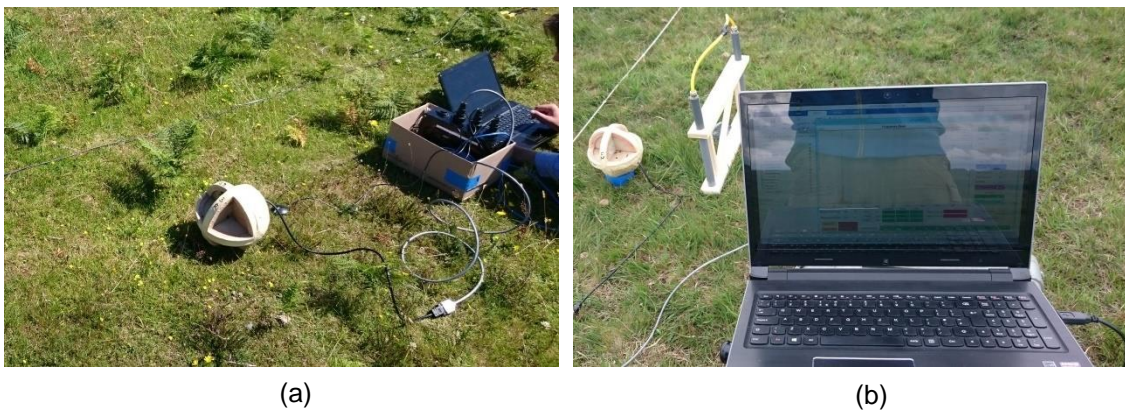
Figure 37 Searching coils tested in the field; (a): Air coils and the acquisition box during field testing; (b): Frequency readings taken during field testing
