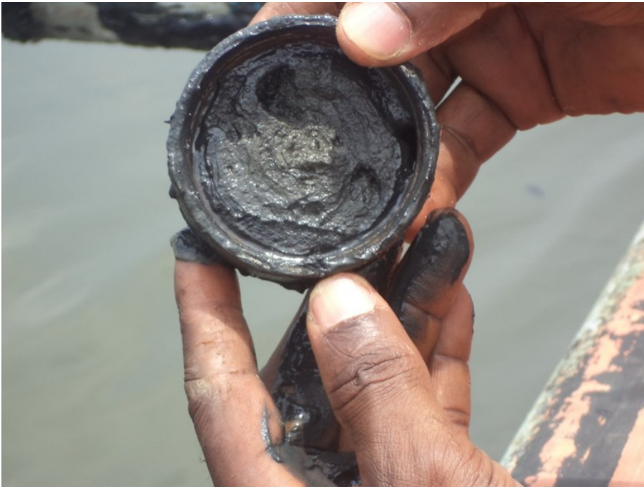
Lid of the locally made sediment corer was opened in order to collect sediment that are trapped inside the grabber so as to redploy it for collection of sediment in other location.
