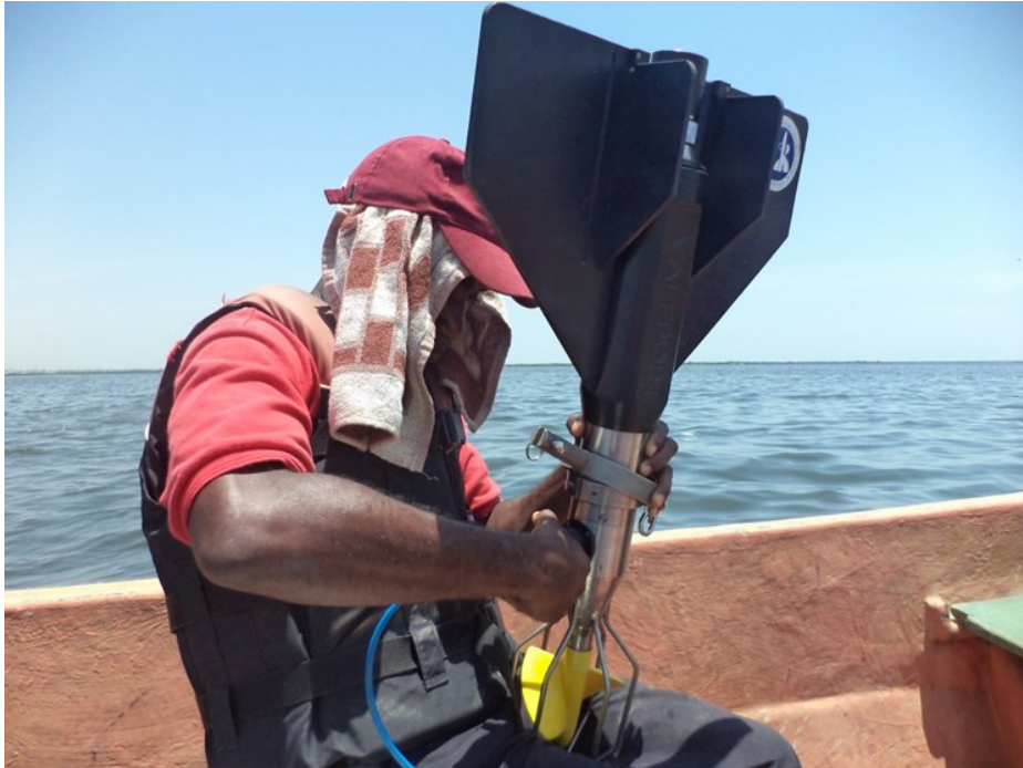
Fixing Valeport current meter for deployment into the Lagos Lagoon
