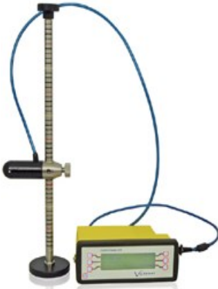
Figure 3.8: Valeport Current Meter (i) Segment that is deployed into water (ii) CDU segment that stored collected data
