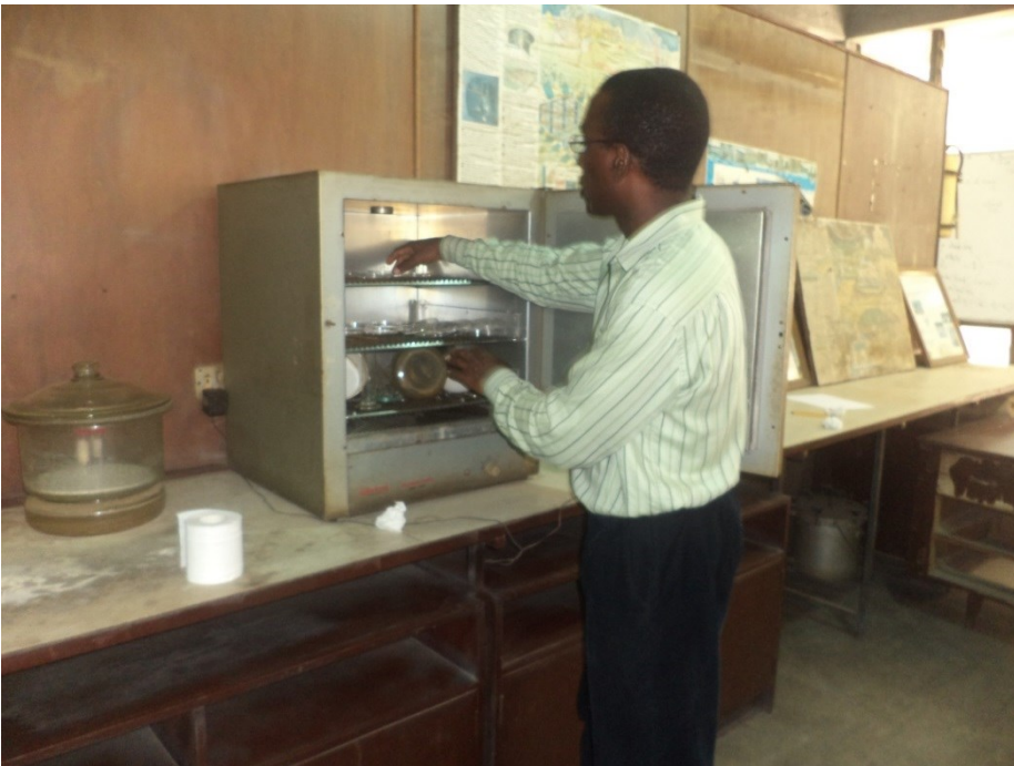
The author putting some sediment samples inside an oven in the laboratory at the Department of Civil and Environmental Engineering, University of Lagos
