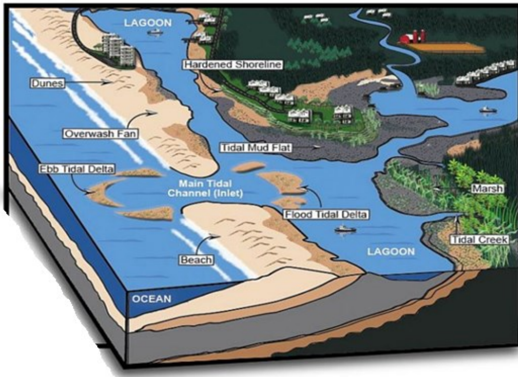
Figure 2.2: Idealized coastal lagoon showing important landforms and characteristics, adapted from (Anthony et al. , 2009)
