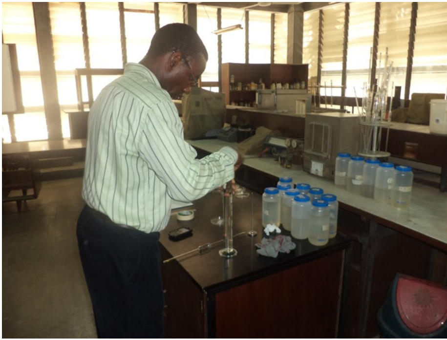
The author while performing Andreasen Pipette experiment at the Department of Civil and Environmental Engineering, University of Lagos
