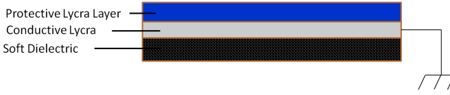
Fig. 2. The sandwich of fabric that constitutes the new dielectric for the sensor. The deformable bottom layer is made with 3D air mesh fabric, the medium layer is made with conductive Lycra that acts as common ground plane for all the taxels. The third layer protects the Lycra and improves the mechanical property of the sensor.
