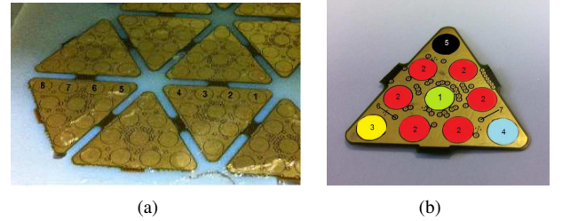
Fig. 15. a) The Figure reports the taxels that were excited during the spatial resolution experiment. The numbers identify the order in which the taxels have been excited. b) Representation of the 10 taxels in the triangle, number code. Taxels with similar temperature drift have been grouped together and represented with the same number. The thermal pads are identified by number 6 and number 7.
