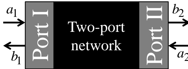
Fig. 4.1. A 2-port network with the input and output signals.
