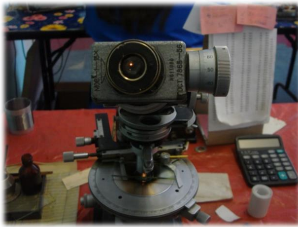
Fig. 1.2. Optical inspection of microwires and their structural features. A piece of equipment from Soviet epoch – still works!
