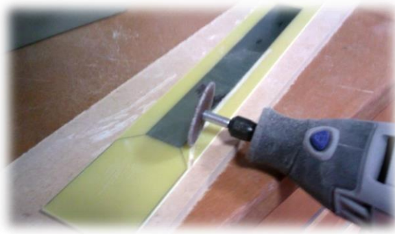
Fig. 3.3. Dog-bone cells being cut from FR4 PCBs with the help of a Dremel rotary cutter.
