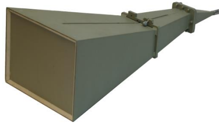
Fig. 4.21. The broadband horn antenna ПГ-23М (0.85 – 17.44 GHz).
