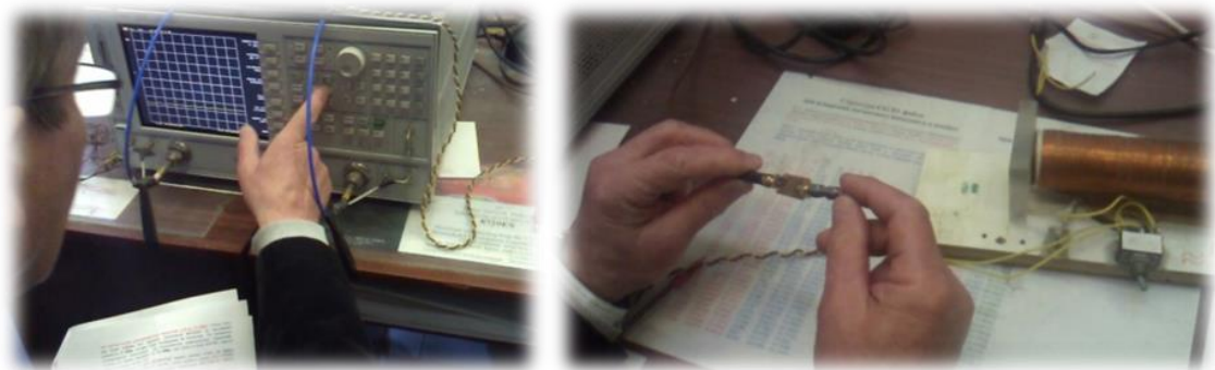
Fig. 1.3. Demonstrations of microwire impedance properties using a VNA and solenoid coil.
