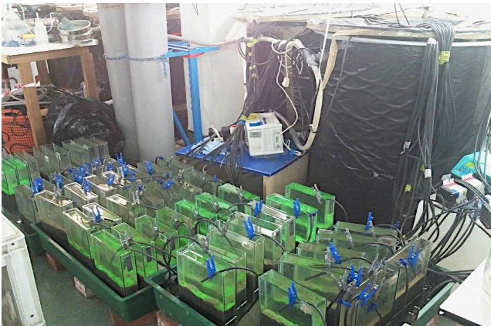
Figure 2.2. Image of the experimental system showing the two header tanks, perisaltic pumps and individual aquairas within a flow through system. Sediment appears green due to the addition of luminophores for bioturbation investigations documented in Chapter 3.
