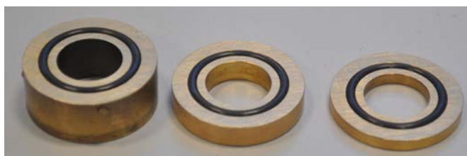
Figure 3.11: ZLC lengthening columns constructed at the University of Plymouth. From left to right, the lengths of the sinters are 10, 5, and 2.7 mm, respectively.
