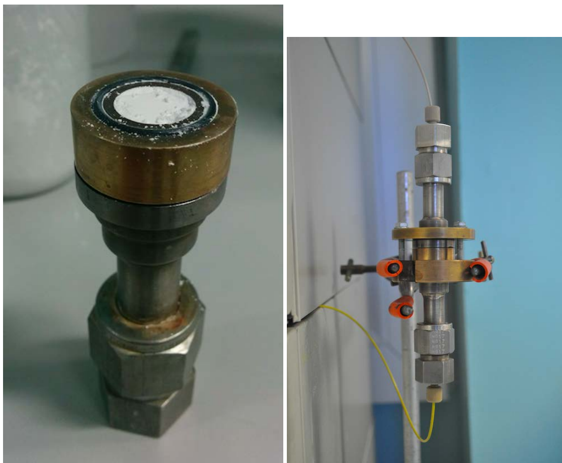
(a) A photograph in the midst of loading the FLC with an FCC sample.
