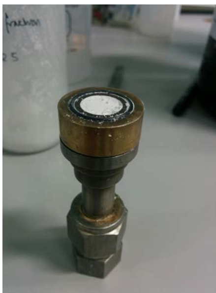
Figure 8.8: A photograph of the loaded FLC before being assembled and attached to the HPLC.
