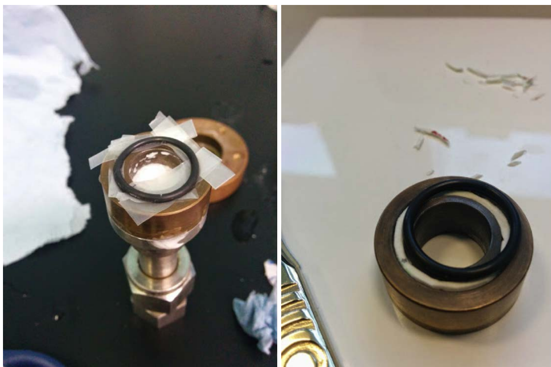
(a) A photograph of the O-ring in a lengthening column being padded out with parafilm.
