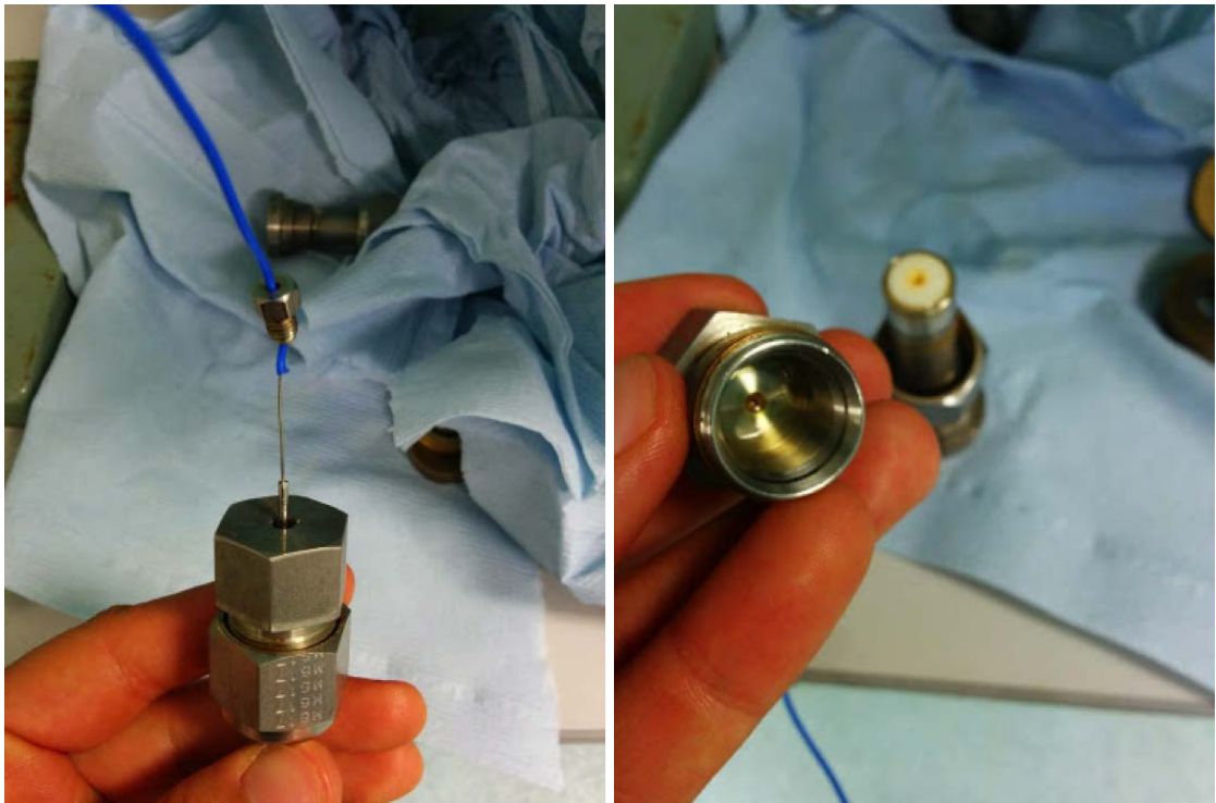
(a) A photograph of the stainless steel capillary stuck in the ZLC.
