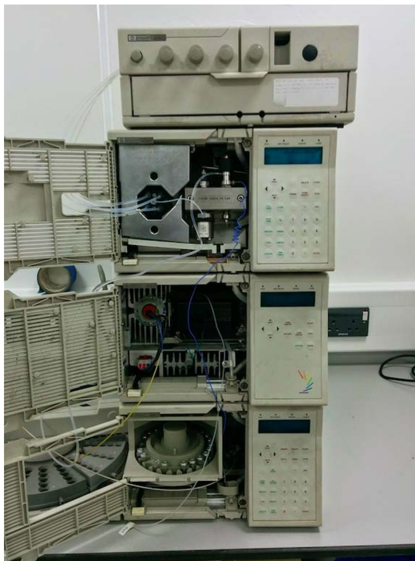
Figure 3.15: A photograph of the Hewlett Packard (now Agilent) HP 1050 series HPLC used throughout this project. The bottom component is the autosampler, the part above is the DAD, the module above that is the pump, and the topmost section is the solvent conditioning module.
