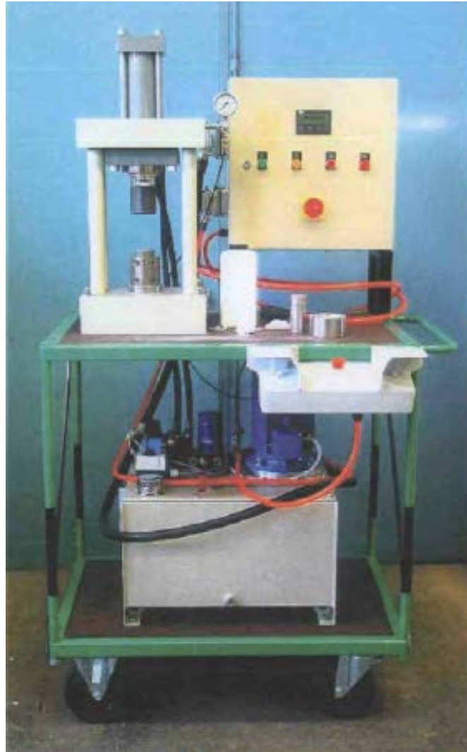
Figure 2.2: A custom-made hydraulic press for tablet compaction that is comprised of a hydraulic unit (on the bottom) with the electronic steering unit (on the top right) and the press-frame with the hydraulic cylinder exerting a force up to 600 kN. The tablets generated are large in size: approximately 4 cm in diameter and 1 cm in thickness. This image is taken from the work of Schoelkopf (2002) .
