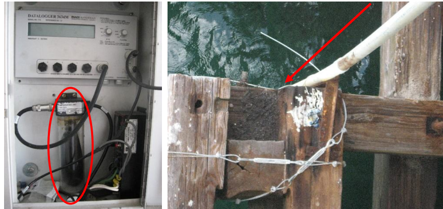
Figure 4.19: Left: Datalogger model 3624M Aanderaa. The red circle shows the balloon used to compensate for the atmospheric pressure. Right: Location of the sensor fixed to Progreso pier.
