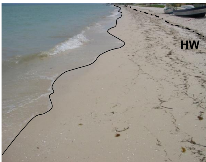
Figure 5.2: Example of the measured shoreline in situ in Progreso, Yucatán. The black solid line indicates the measured shoreline. The black dotted line shows the mark of the last high water.
