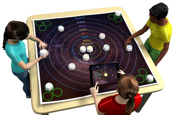
Figure 1: Concept Cellulo activities: Left: Robots simulate planets orbiting the sun. The learners can move the planets to alter their orbits or even attempt to remove the sun. Right: Robots represent atoms with Brownian motion. The learners can directly interact with atoms to change their temperature or add/remove atoms to experiment with conditions under which molecules form and break down.
