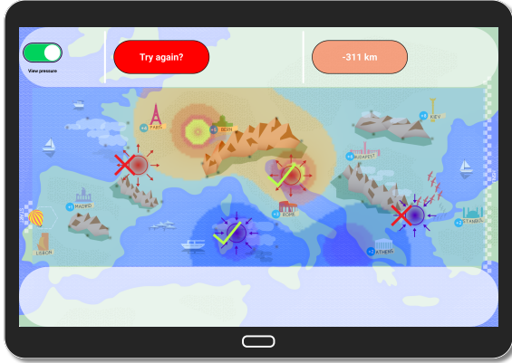
Figure 7: Screen capture of the Windfield activity application running on the tablet. Position of the balloon is synchronized with the position of the robot on the real map. Low and high pressure areas are represented in blue and red respectively.
