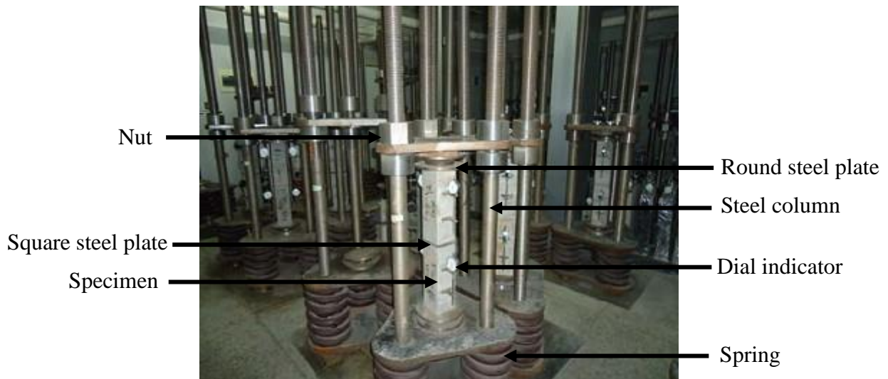
Fig.7 Processes of creep test
