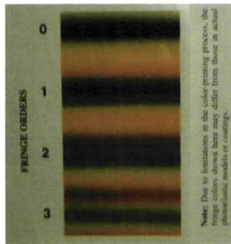
Figure 5.10 Colour scale (VISHAY® PhotoStress Tech Note )
