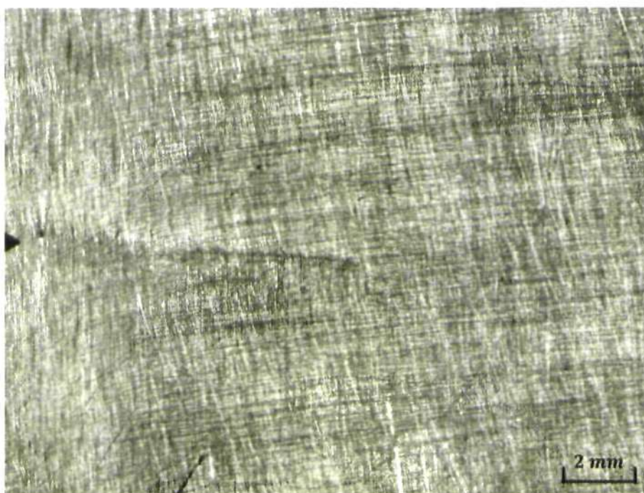
Figure 4.37 Random patterns of scratches applied to the surface of the specimen ALCT-R01.
