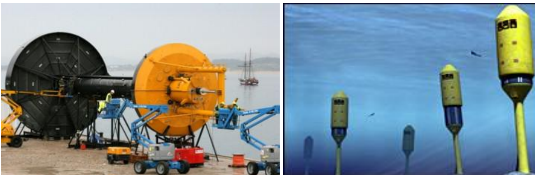
Figure 2.11 The floating PowerBuoy prototype (left) and submerged Archimedes Wave Swing (right). Sources: Ocean Power Technologies Inc (2014) and AWS Ocean Energy (2015)
