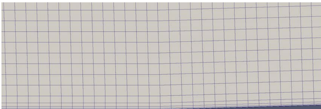
Figure 5.3: A magnified view of the near-wall discretisation for the mesh generated using the merging technique, shown in Figure 5.2, with additional near-wall layers included using snappyHexMesh .
