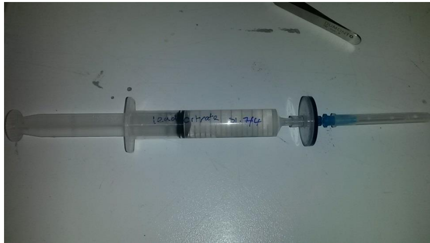
Figure 2.11 A syringe of Reynold's lead citrate with attached filter and needle ready for use.
