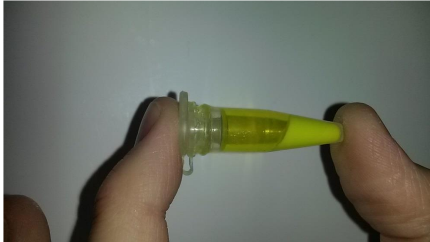
Figure 2.8 the same tube having been centrifuged. The desired supernatant is the clearer yellow on the left.
