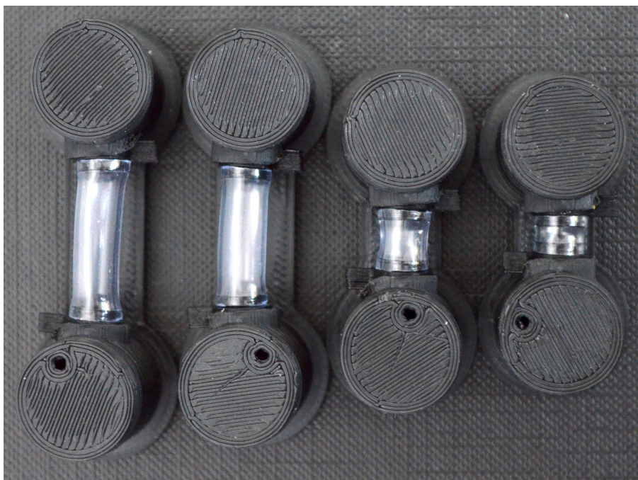
Figure 6.2: A photograph of the receptacles set up with different tube lengths to investigate the effect on memristance. Shown are connecting tube lengths of 2.5mm, 5mm, 15mm, and 20mm.
