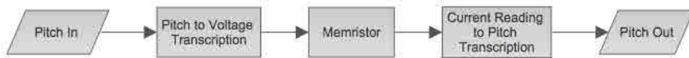
Figure 5.12: A flow diagram of the basic mapping approach for generating pitches using a memristor.
