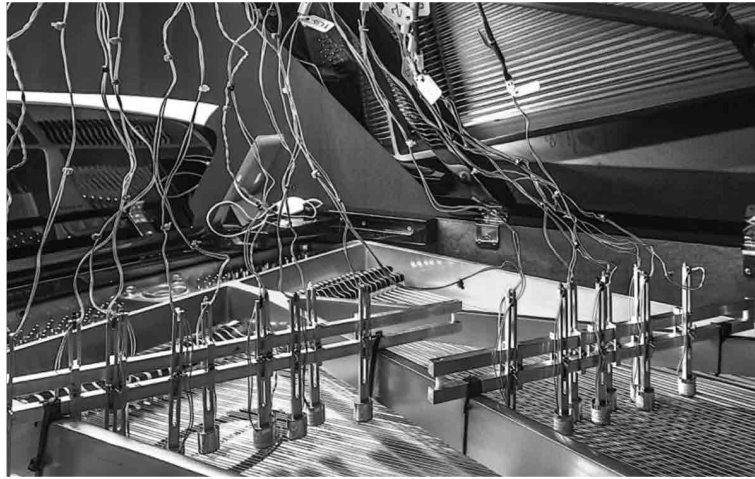
Figure 5.20: A photograph of twenty-four electromagnets furnished above the strings of a grand piano.
