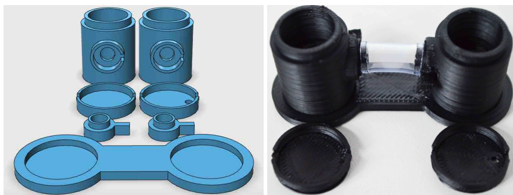
Figure 6.1: A screenshot (left) and photograph (right) of the receptacle. Shown is two identical growth chambers, two lids (one with and one without an air hole), two conductive electrode collars and a 10mm base.
