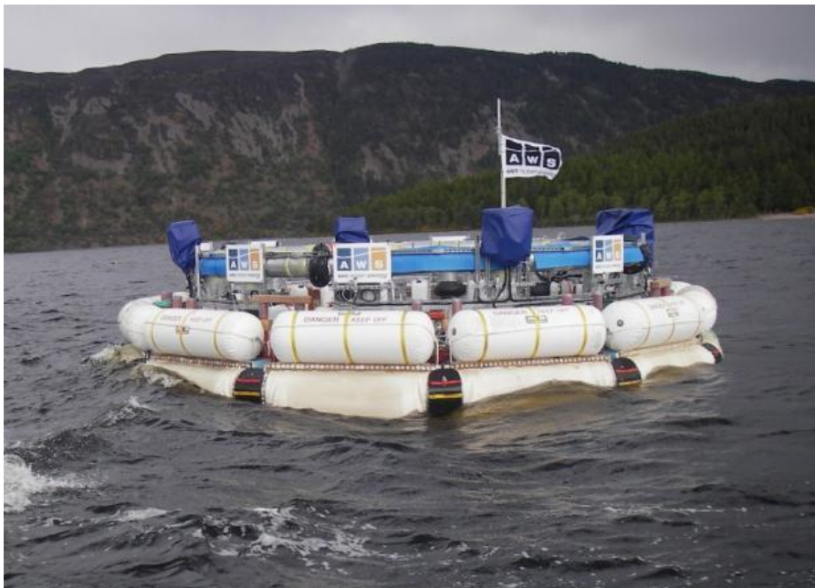
Figure 1.14: 1:9 Scale model of the AWS-III under test on Loch Ness, June 2010
