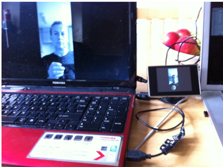
Illustration 19. 30-line digital image displayed on a mini television monitor (image by the author).
