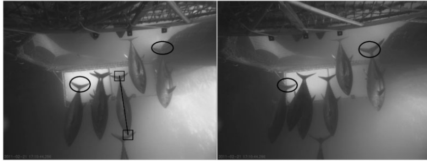
Figure 2. A stereo pair of frames in which snout and tail of the fish to be measured is shown in the left frame with black squares, where the squares represent the image region used for template matching. Note that due to different perspectives of the camera, the background changes significantly between the two images. Two sample tails in each frame are marked with black ellipses to illustrate this effect.
