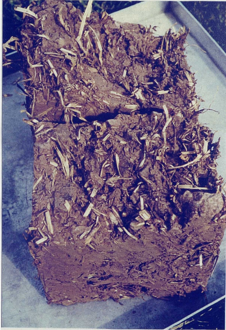
plate 3.1 Fibre pull- out (courtesy of Robert Saxton)
